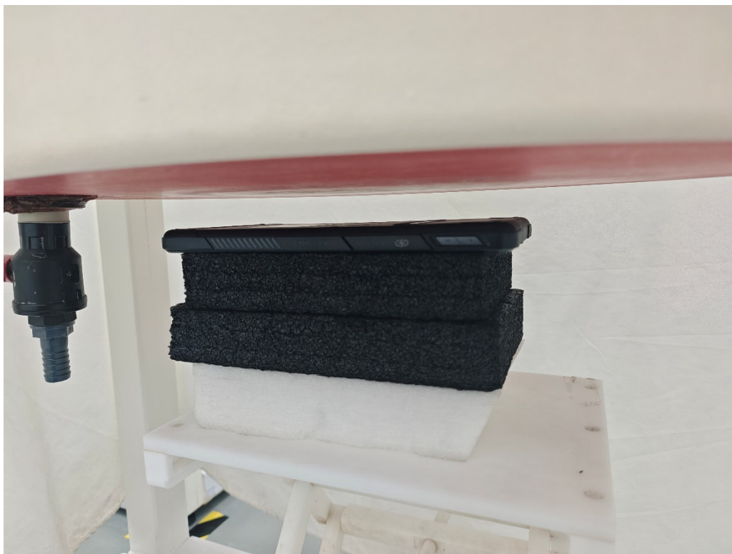
Picture 7: Back Side, the distance from EUT to the bottom of the Phantom is 25mm
