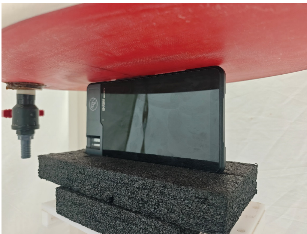
Picture 4: Right Edge, the distance from EUT to the bottom of the Phantom is 0mm
