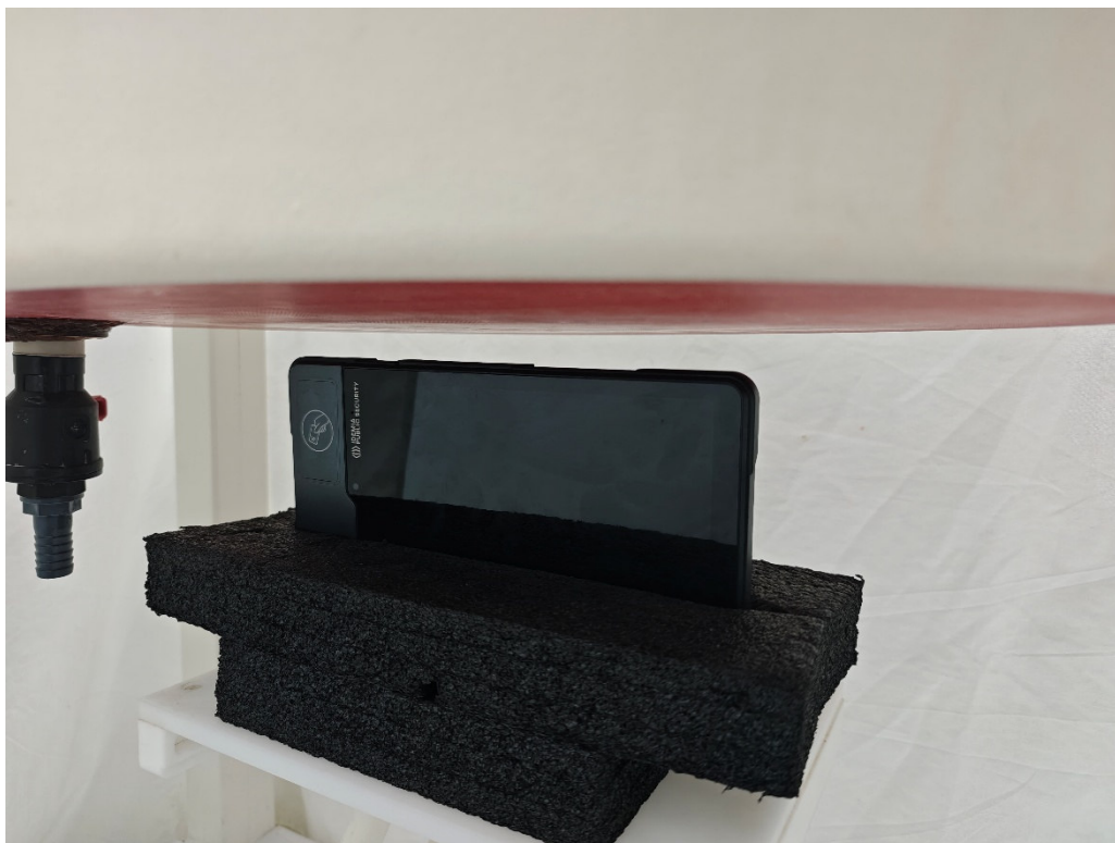
Picture 8: Right Edge, the distance from EUT to the bottom of the Phantom is 17mm
