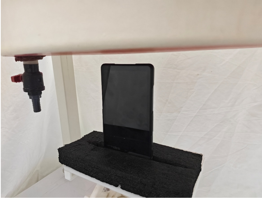
Picture 9: Bottom Edge, the distance from EUT to the bottom of the Phantom is 21mm
