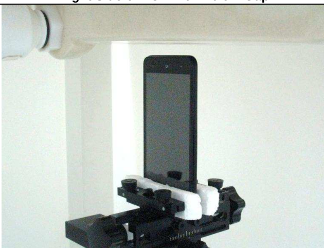
Right Side of EUT with 1.0 cm Gap
