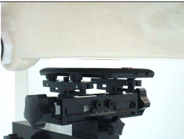
Rear Face of EUT with 1.0 cm Gap
