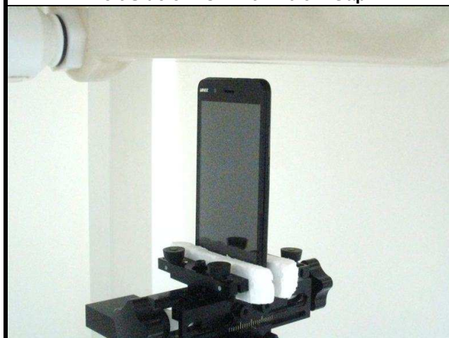
Left Side of EUT with 1.0 cm Gap
