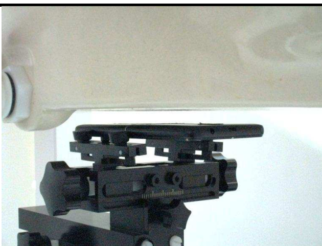
Rear Face of EUT with 1.0 cm Gap
