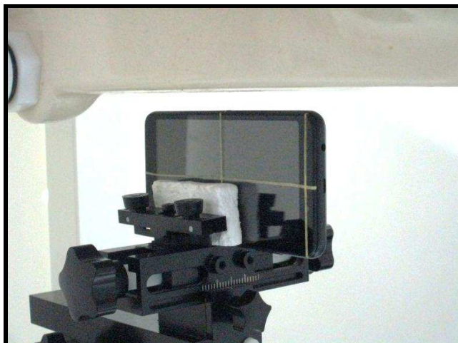
Left Side of EUT with 1.0 cm Gap
