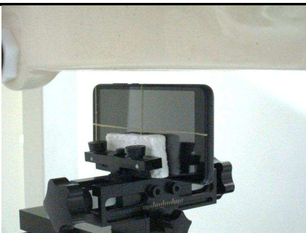
Right Side of EUT with 1.0 cm Gap
