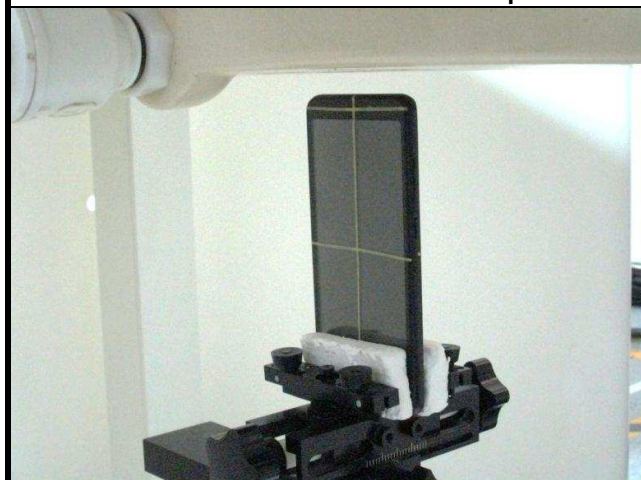
Top Side of EUT with 1.0 cm Gap
