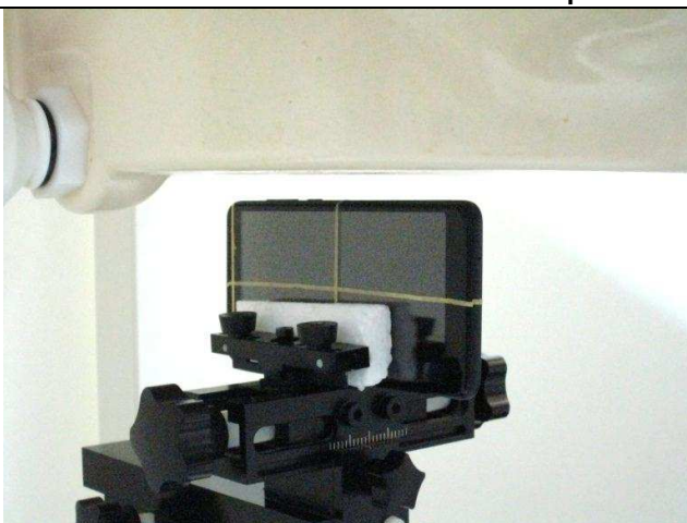
Right Side of EUT with 1.0 cm Gap
