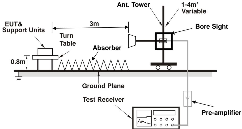
\* : depends on the EUT height and the antenna 3dB beamwidth both, refer to section 7.3 of CISPR 16-2-3.
