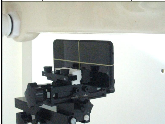
Left Side of EUT with 1.0 cm Gap
