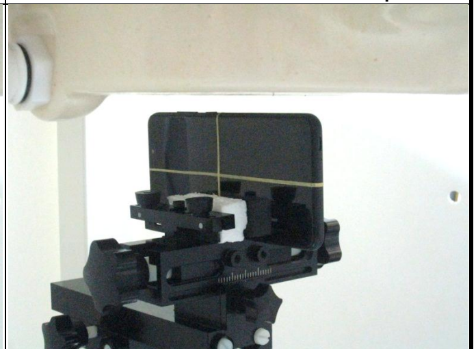
Right Side of EUT with 1.0 cm Gap
