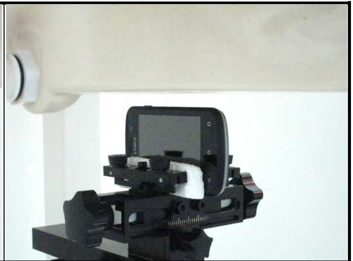
Right Side of EUT with 1.0 cm Gap
