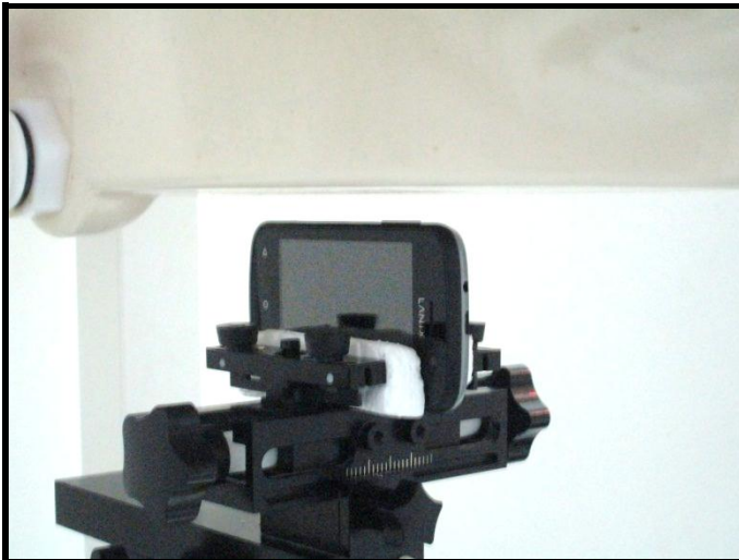
Left Side of EUT with 1.0 cm Gap
