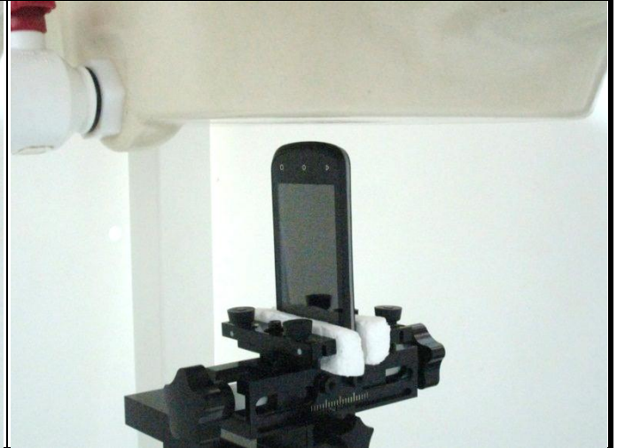
Bottom Side of EUT with 1.0 cm Gap
