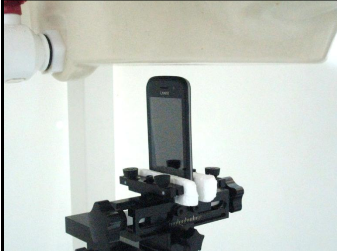
Top Side of EUT with 1.0 cm Gap
