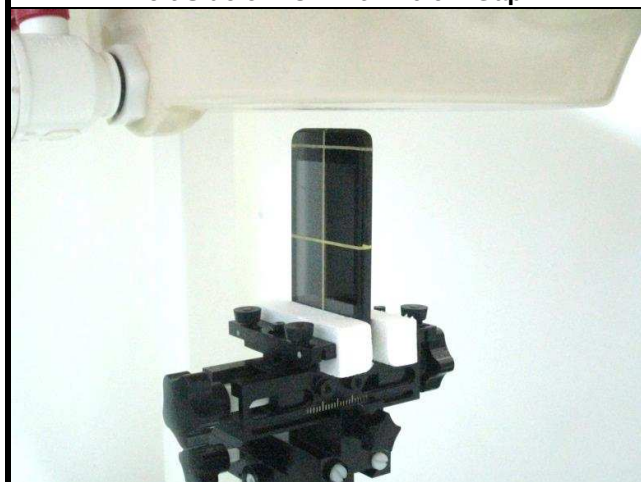
Top Side of EUT with 1.0 cm Gap
