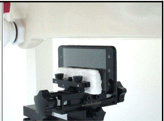
Right Side of EUT with 1.0 cm Gap
