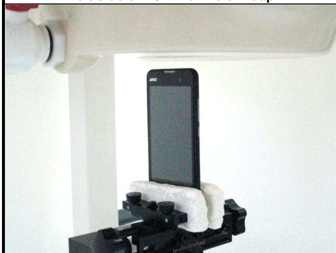
Top Side of EUT with 1.0 cm Gap
