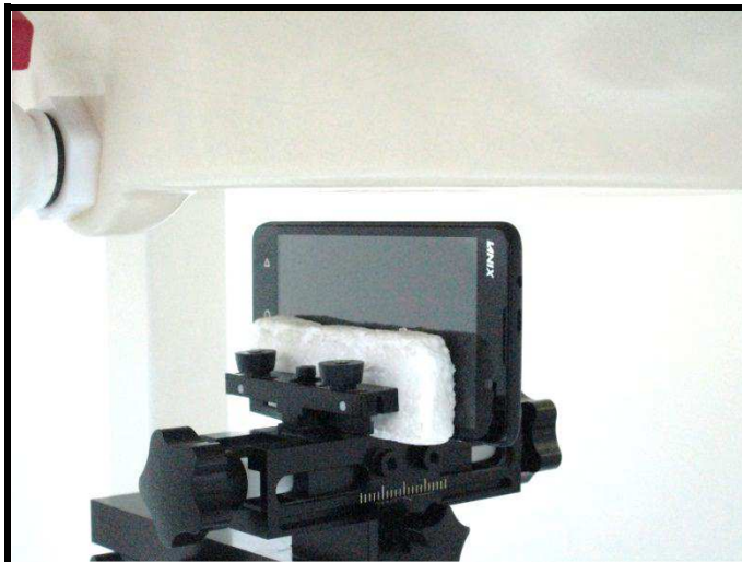
Left Side of EUT with 1.0 cm Gap
