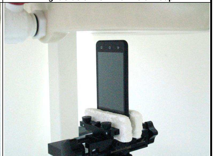
Bottom Side of EUT with 1.0 cm Gap
