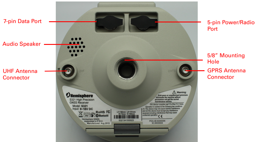
Figure 2-1: S321 ports and connectors
