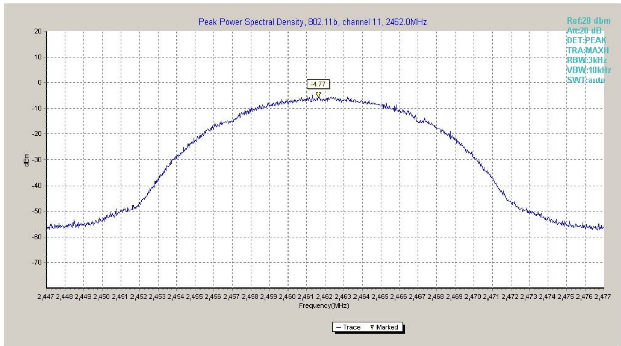
Fig.A.3.3 Power Spectral Density (802.11b, Ch 11)
