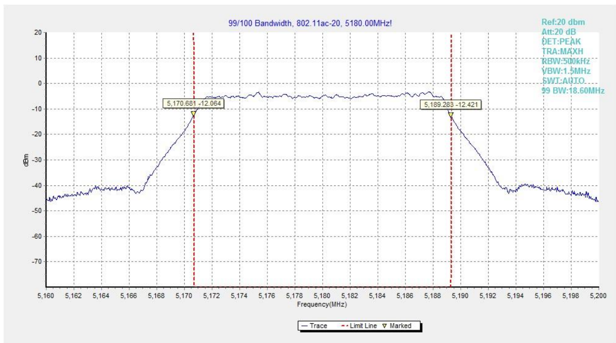
Fig.62 99% Occupied bandwidth (802.11ac-HT20, 5180MHz)
