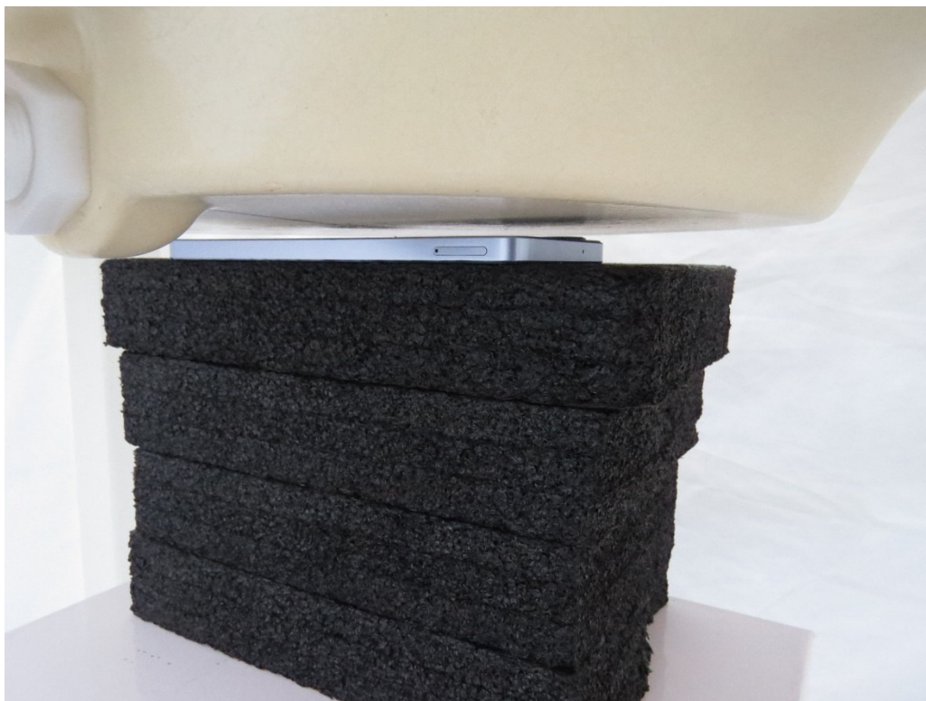
Picture 5: Back Side, the distance from EUT to the bottom of the Phantom is 5mm
