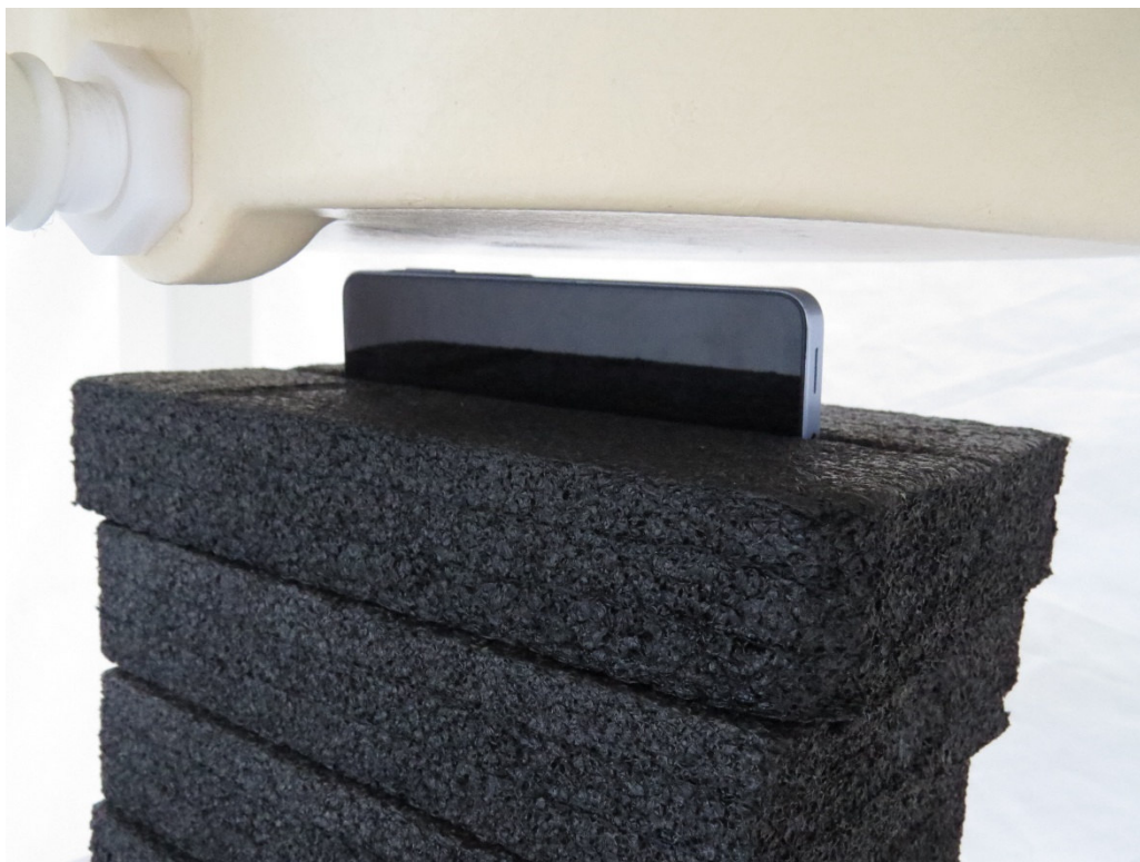
Picture 20: Right Edge, the distance from EUT to the bottom of the Phantom is 8mm
