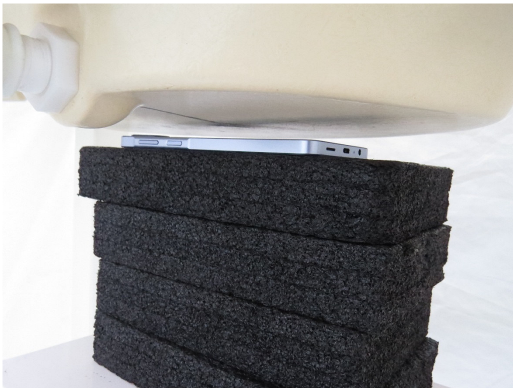
Picture 11: Back Side, the distance from EUT to the bottom of the Phantom is 10mm
