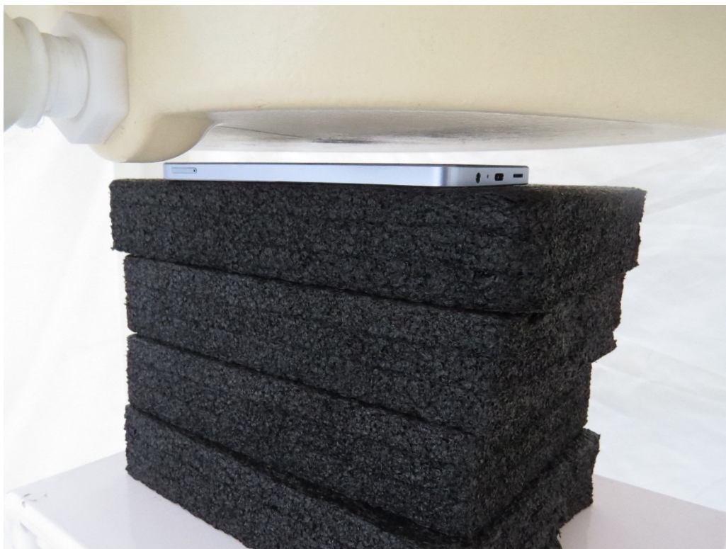
Picture 12: Front Side, the distance from EUT to the bottom of the Phantom is 10mm
