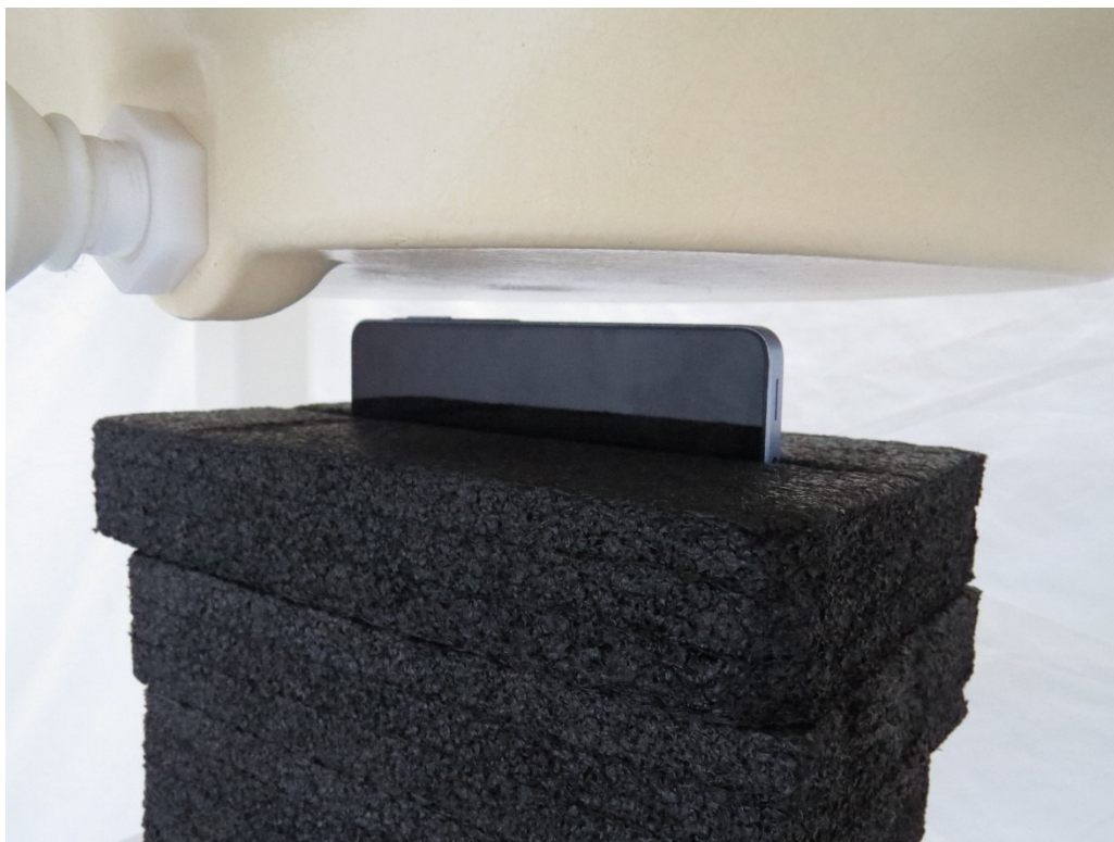
Picture 14: Right Edge, the distance from EUT to the bottom of the Phantom is 10mm
