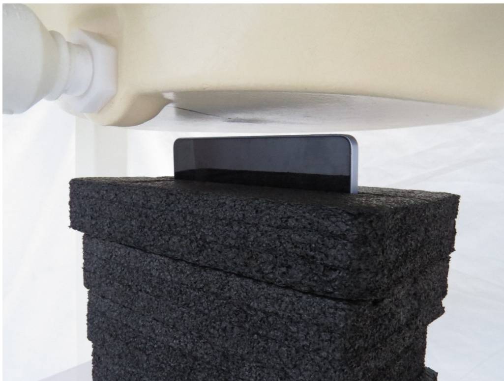
Picture 13: Left Edge, the distance from EUT to the bottom of the Phantom is 10mm
