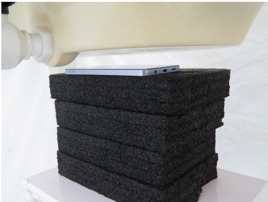
Picture 18: Front Side, the distance from EUT to the bottom of the Phantom is 19mm
