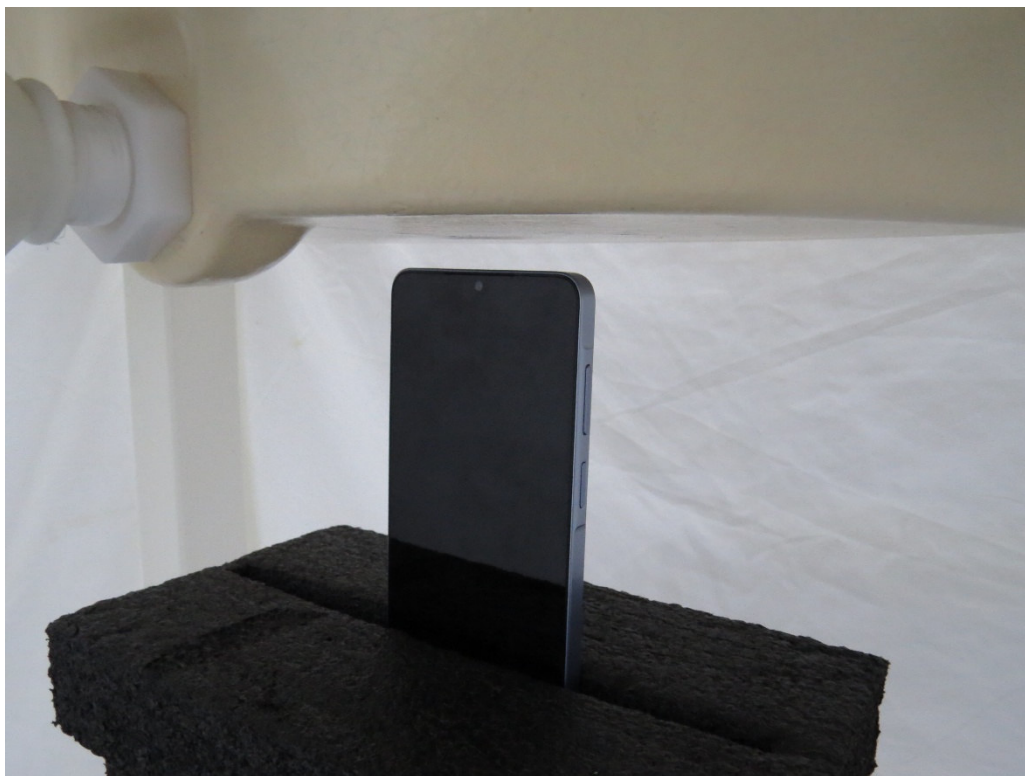
Picture 15: Top Edge, the distance from EUT to the bottom of the Phantom is 10mm
