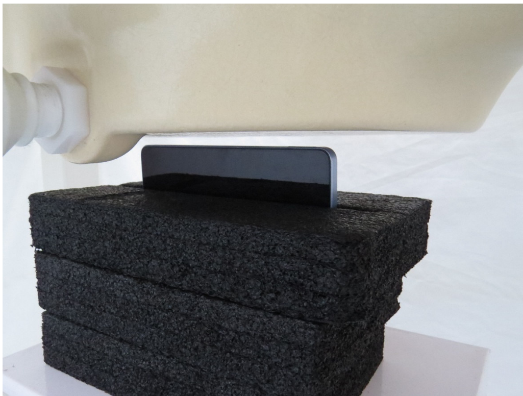
Picture 7: Left Edge, the distance from EUT to the bottom of the Phantom is 5mm
