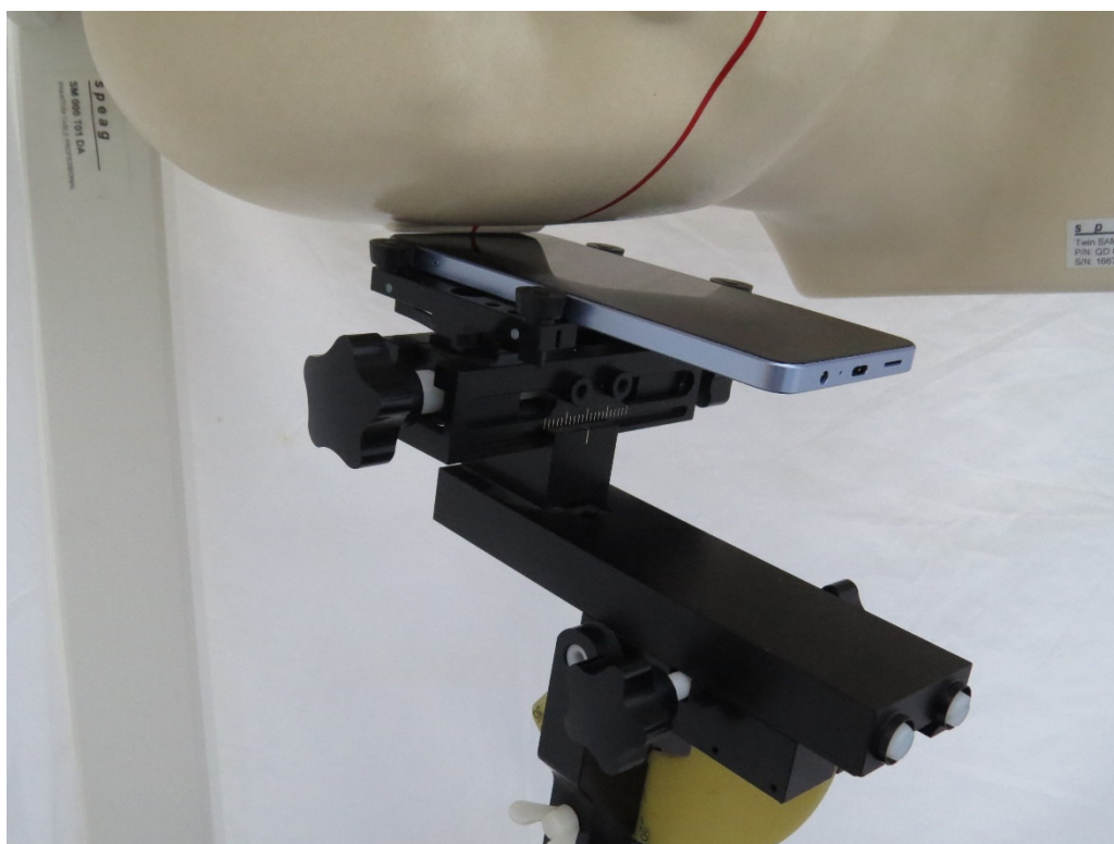
Picture 4: Right Tilt 15 Degree Position
