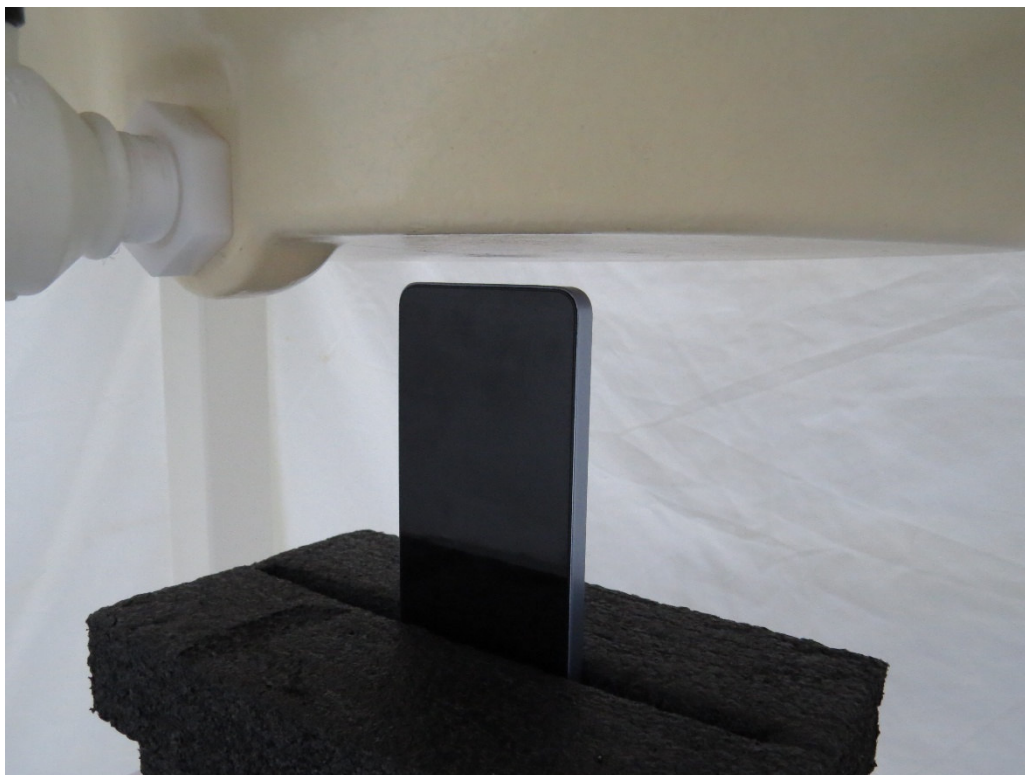
Picture 16: Bottom Edge, the distance from EUT to the bottom of the Phantom is 10mm
