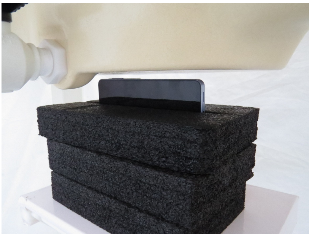
Picture 8: Right Edge, the distance from EUT to the bottom of the Phantom is 5mm
