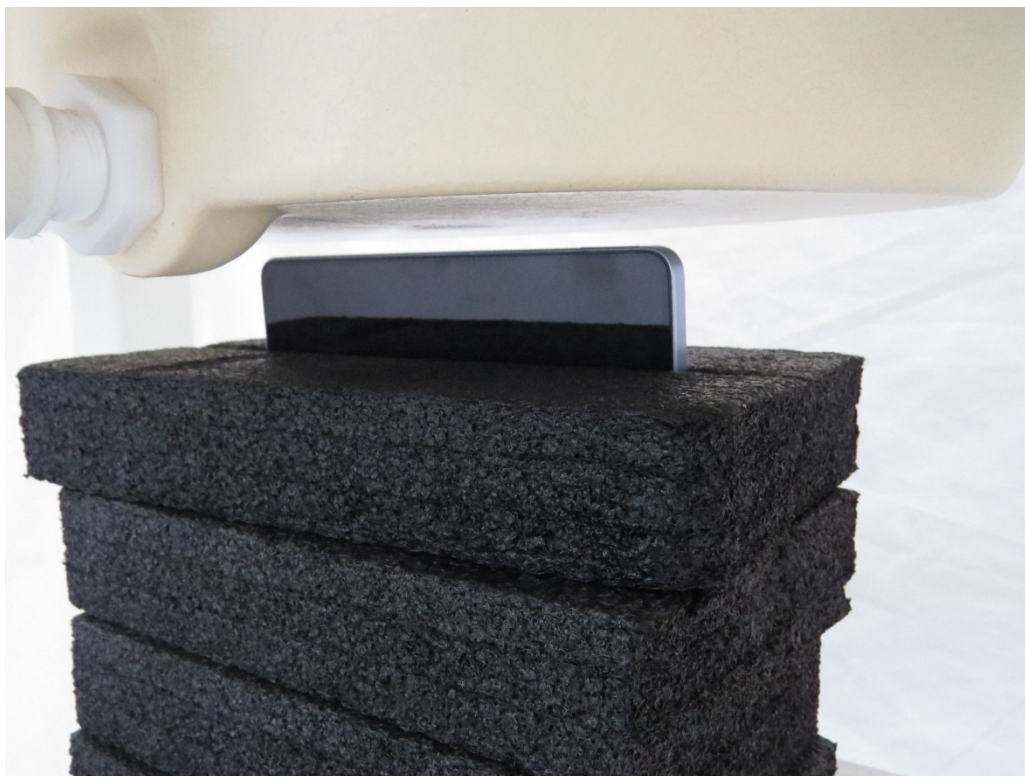
Picture 19: Left Edge, the distance from EUT to the bottom of the Phantom is 7mm
