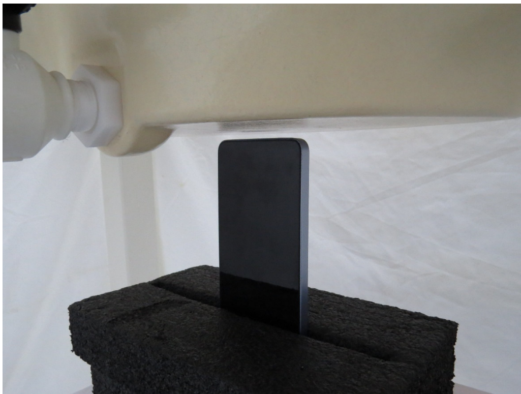
Picture 10: Bottom Edge, the distance from EUT to the bottom of the Phantom is 5mm
