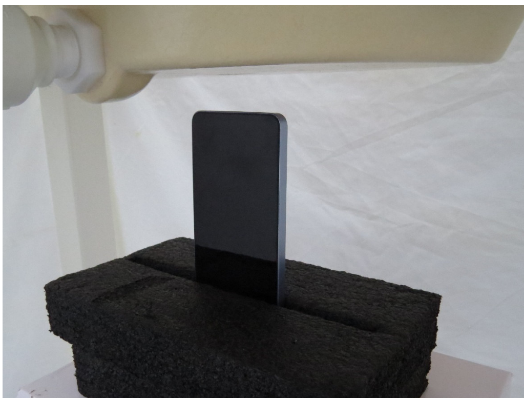
Picture 22: Bottom Edge, the distance from EUT to the bottom of the Phantom is 26mm
