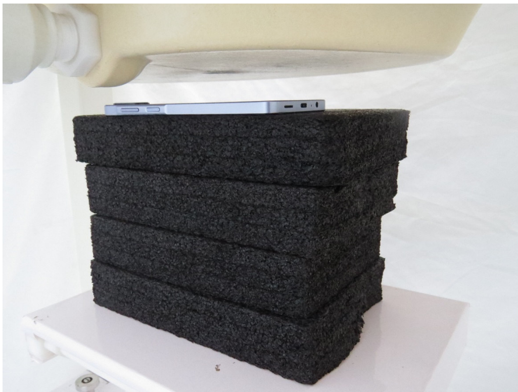
Picture 17: Back Side, the distance from EUT to the bottom of the Phantom is 26mm
