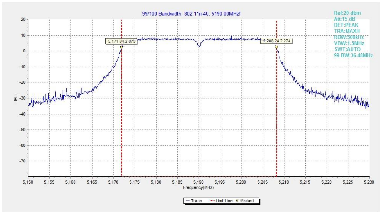
Fig.98 99% Occupied bandwidth (802.11n-HT40, 5190MHz)
