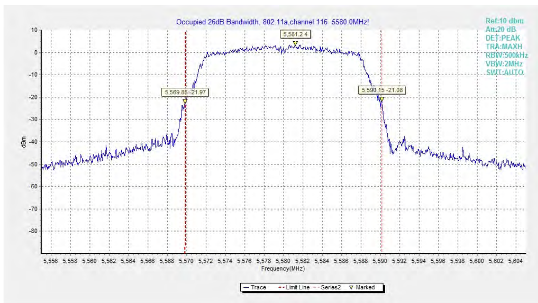
Fig.8 Occupied 26dB Bandwidth (802.11a, 5580MHz)
