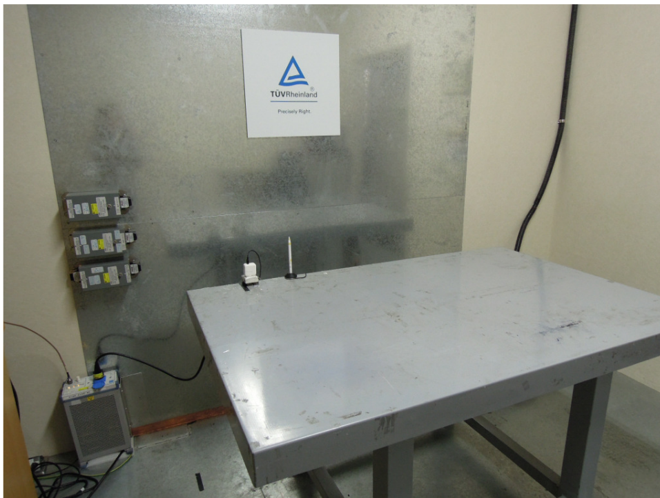
Photograph 7: Set-up for Mains Conducted testing (Front view)
