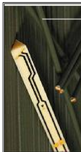
Inside View of SN11/09 EP100 E-field Probe Half of half to
