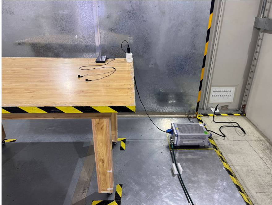
Conducted Emissions (Left View)
