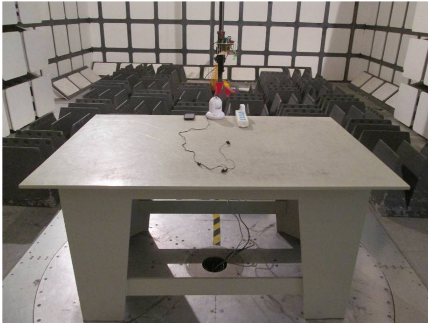
Radiated Emissions – Front View (Above 1 GHz)
