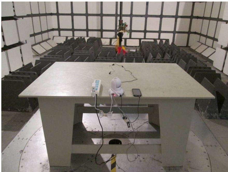
Radiated Emissions – Rear View (Above 1 GHz)
