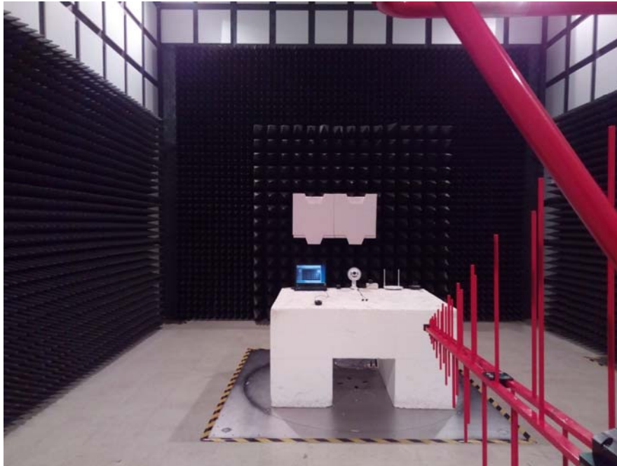
Radiated Emissions – Front View (Below 1 GHz)
