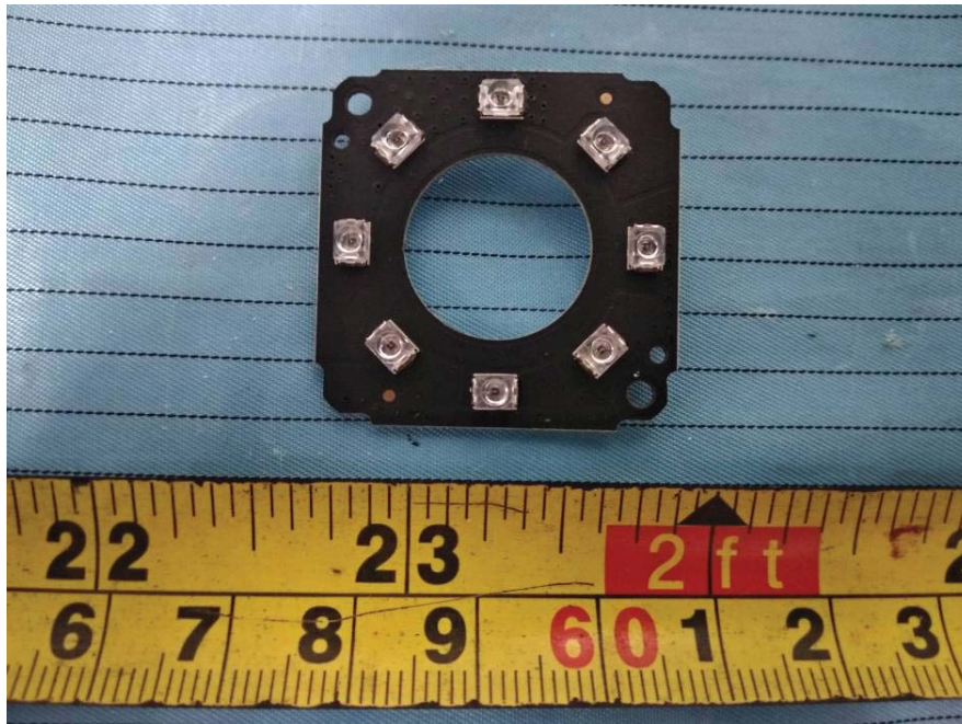
EUT – LED Board Top View
