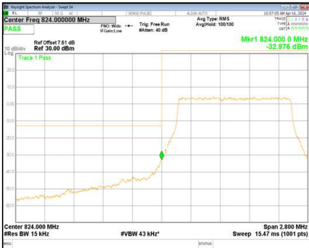
Band5 QPSK BW=1.4MHz Channel=20643 RB Size=6 Position=#0
