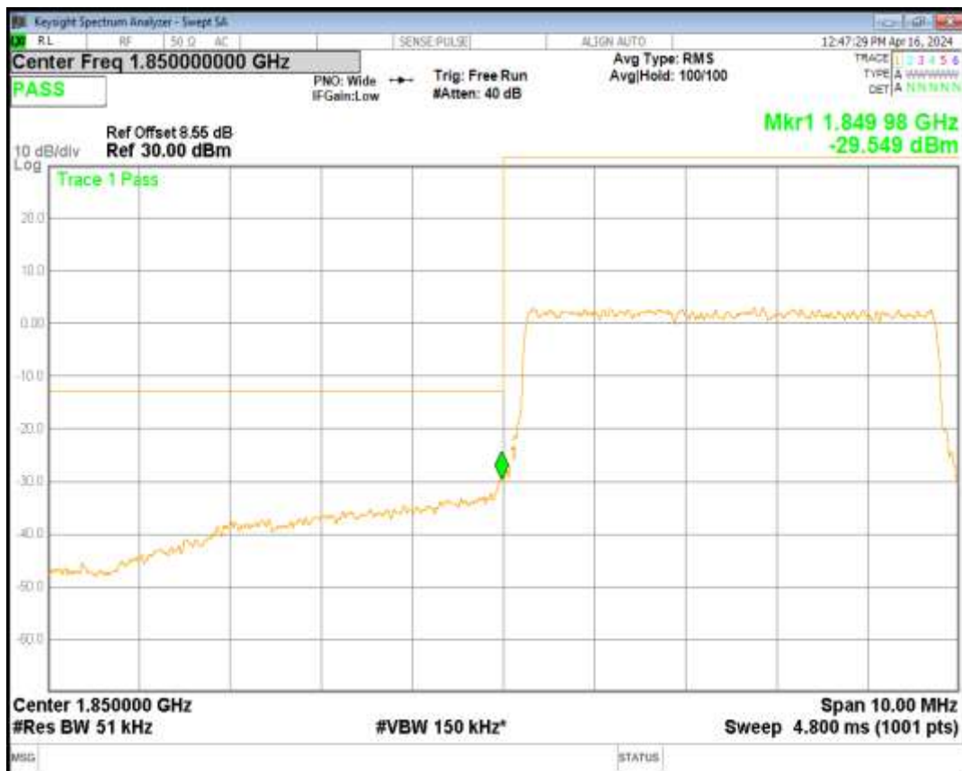
Band2 QPSK BW=5MHz Channel=19175 RB Size=25 Position=#0
