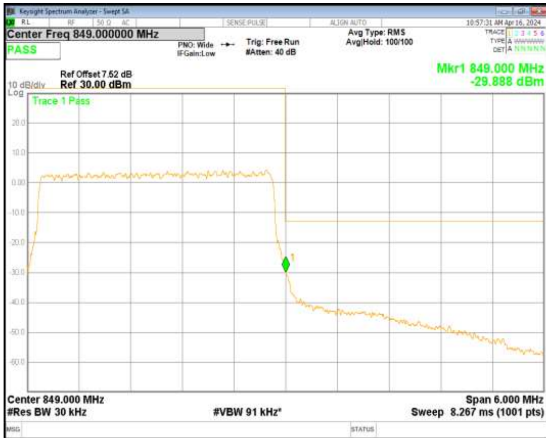
Band5 QPSK BW=5MHz Channel=20425 RB Size=25 Position=#0
