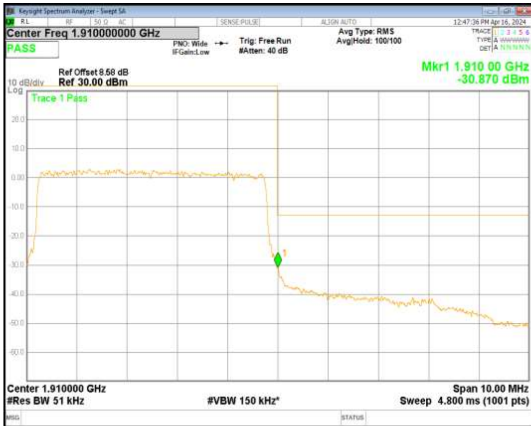
Band2 QPSK BW=10MHz Channel=19150 RB Size=50 Position=#0
