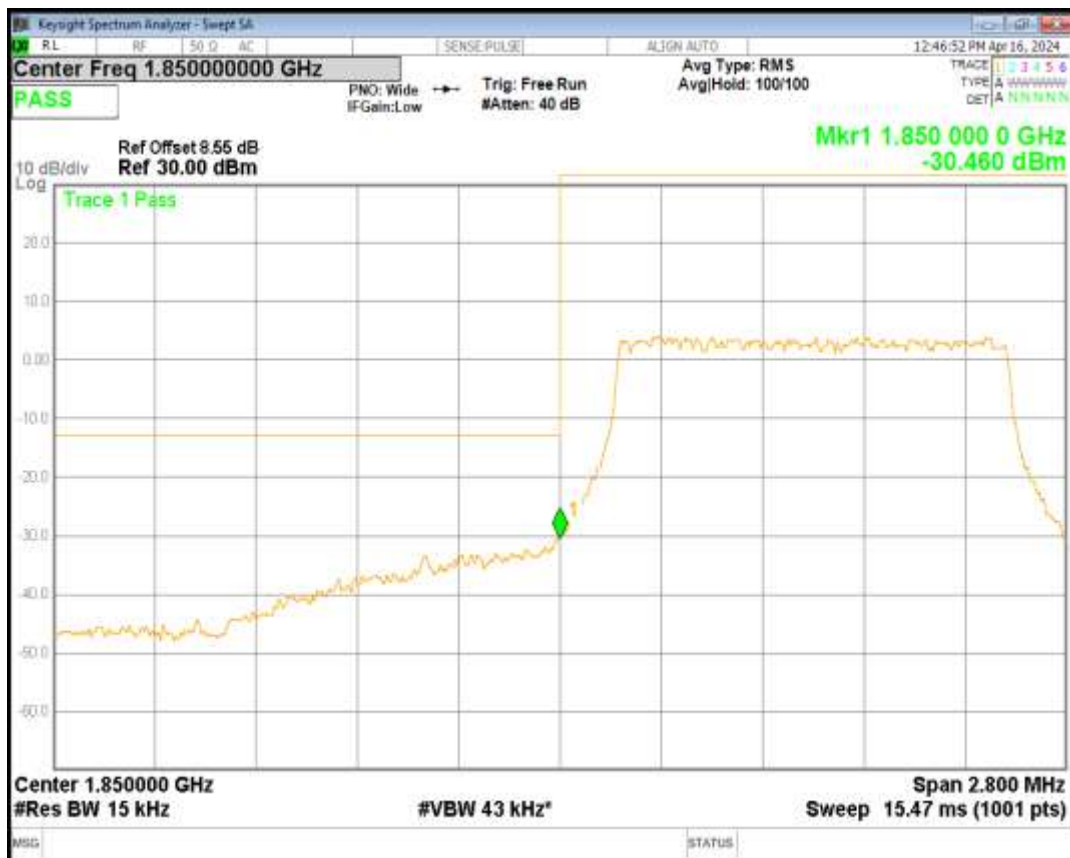
Band2 QPSK BW=1.4MHz Channel=19193 RB Size=6 Position=#0
