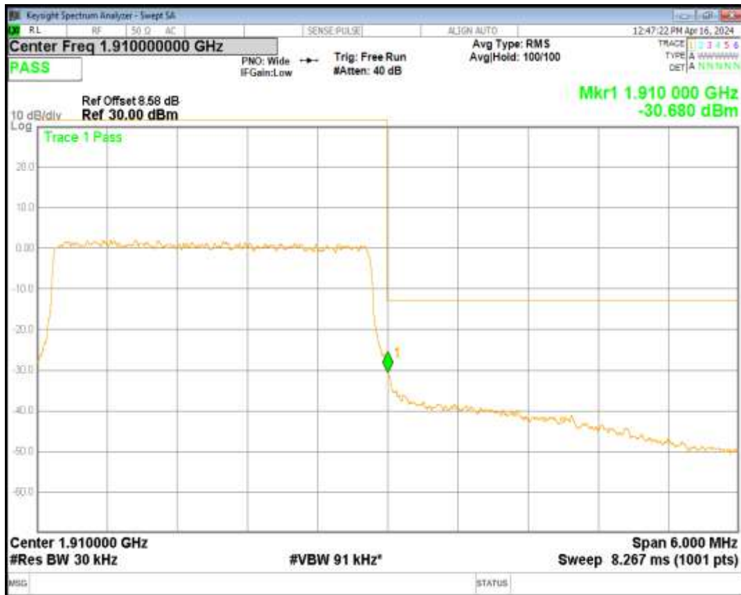
Band2 16QAM BW=5MHz Channel=18625 RB Size=25 Position=#0
