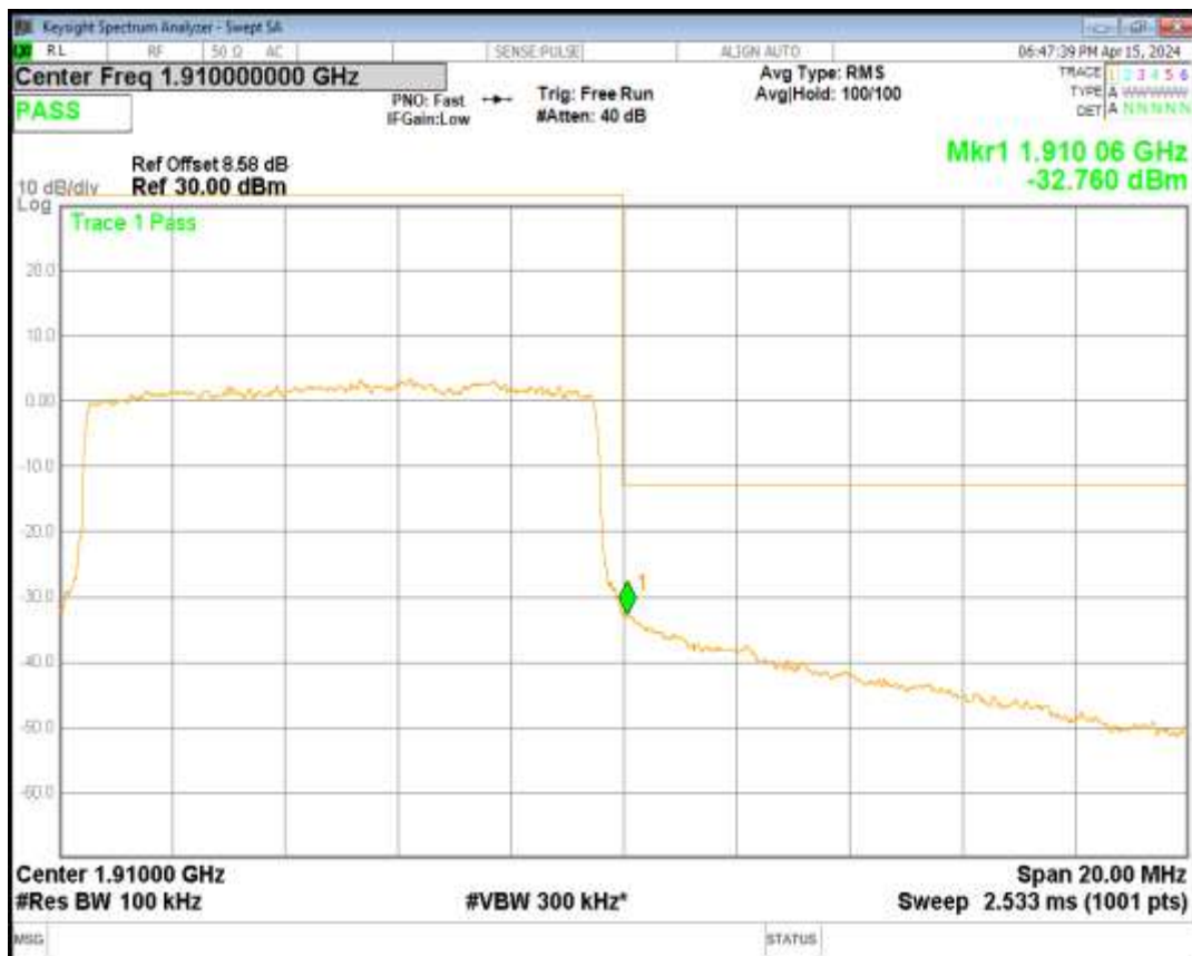
Band2 QPSK BW=10MHz Channel=18650 RB Size=50 Position=#0
