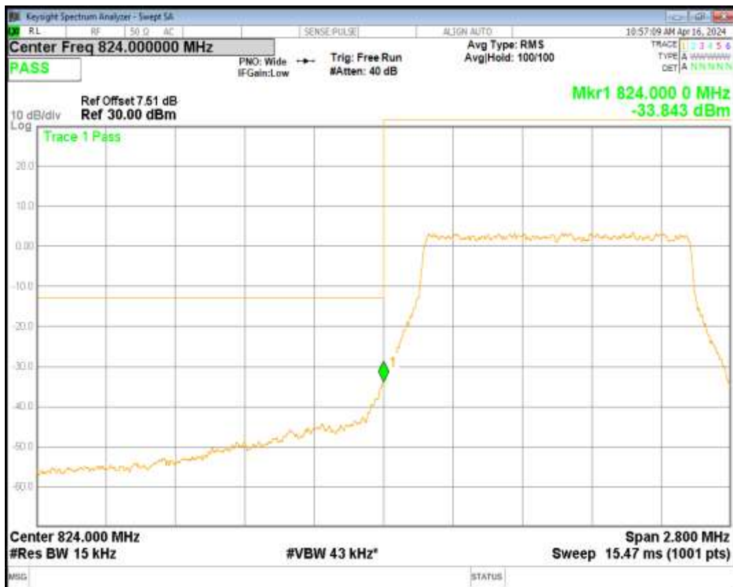
Band5 16QAM BW=1.4MHz Channel=20643 RB Size=6 Position=#0
