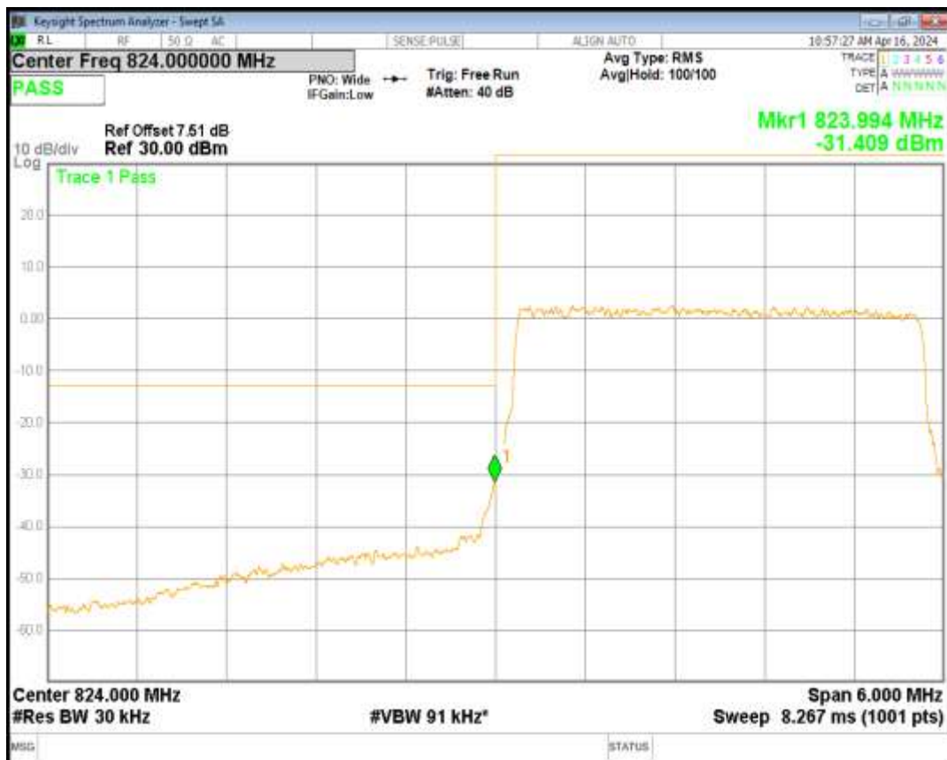
Band5 16QAM BW=3MHz Channel=20635 RB Size=15 Position=#0
