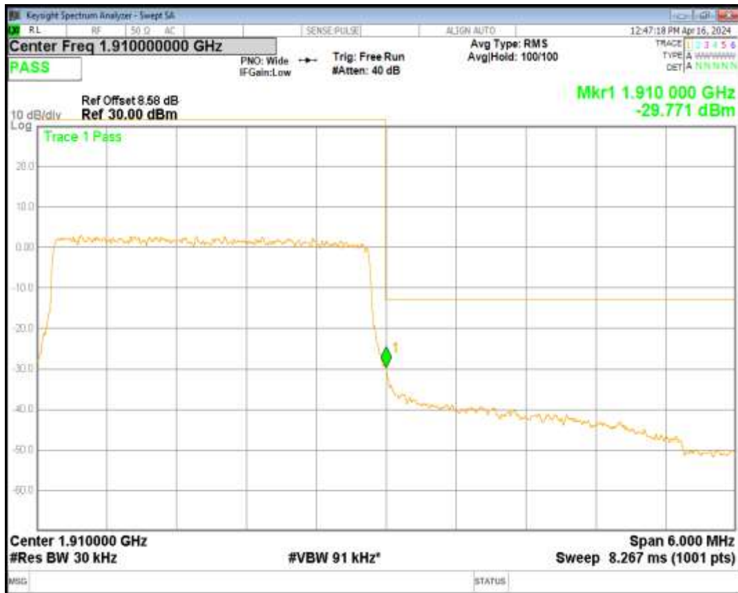
Band2 QPSK BW=5MHz Channel=18625 RB Size=25 Position=#0
