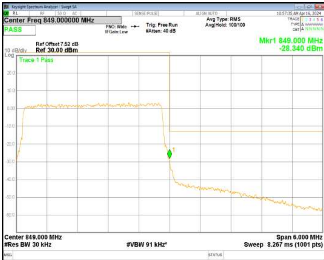
Band5 16QAM BW=5MHz Channel=20425 RB Size=25 Position=#0
