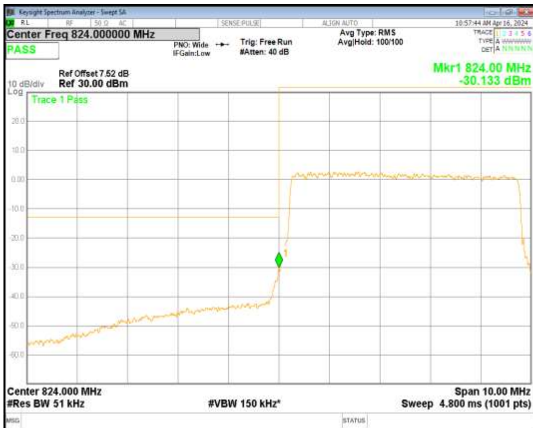
Band5 16QAM BW=5MHz Channel=20625 RB Size=25 Position=#0
