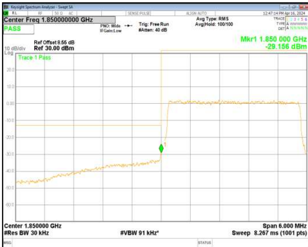
Band2 16QAM BW=3MHz Channel=19185 RB Size=15 Position=#0
