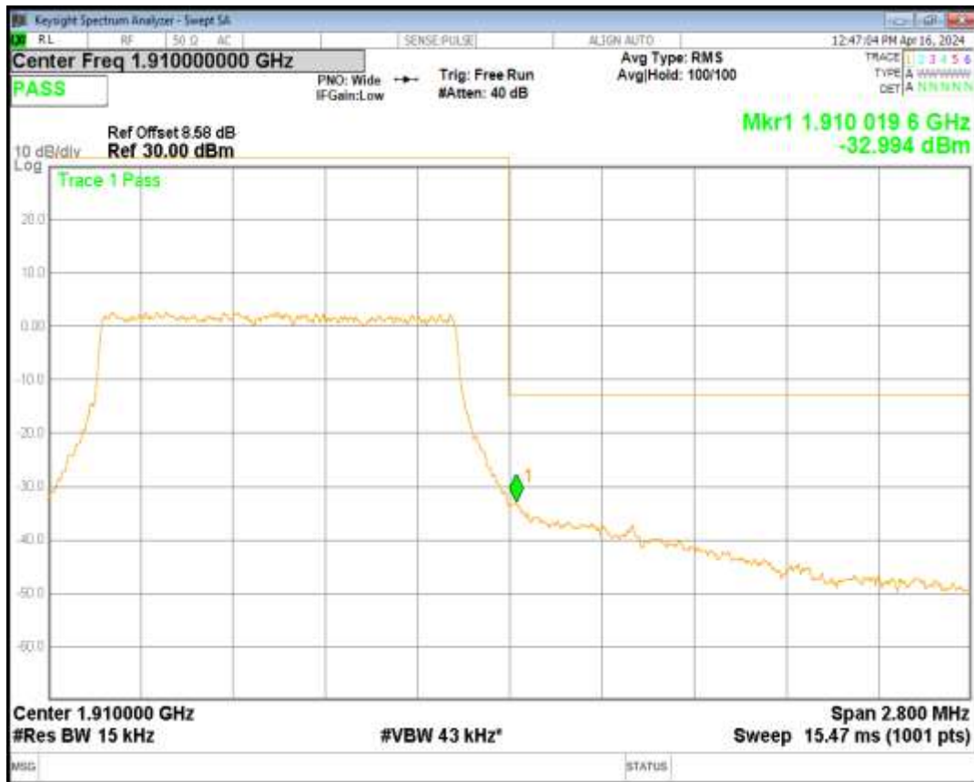
Band2 16QAM BW=3MHz Channel=18615 RB Size=15 Position=#0
