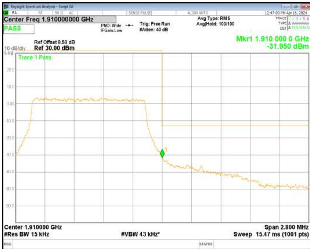
Band2 QPSK BW=3MHz Channel=18615 RB Size=15 Position=#0
