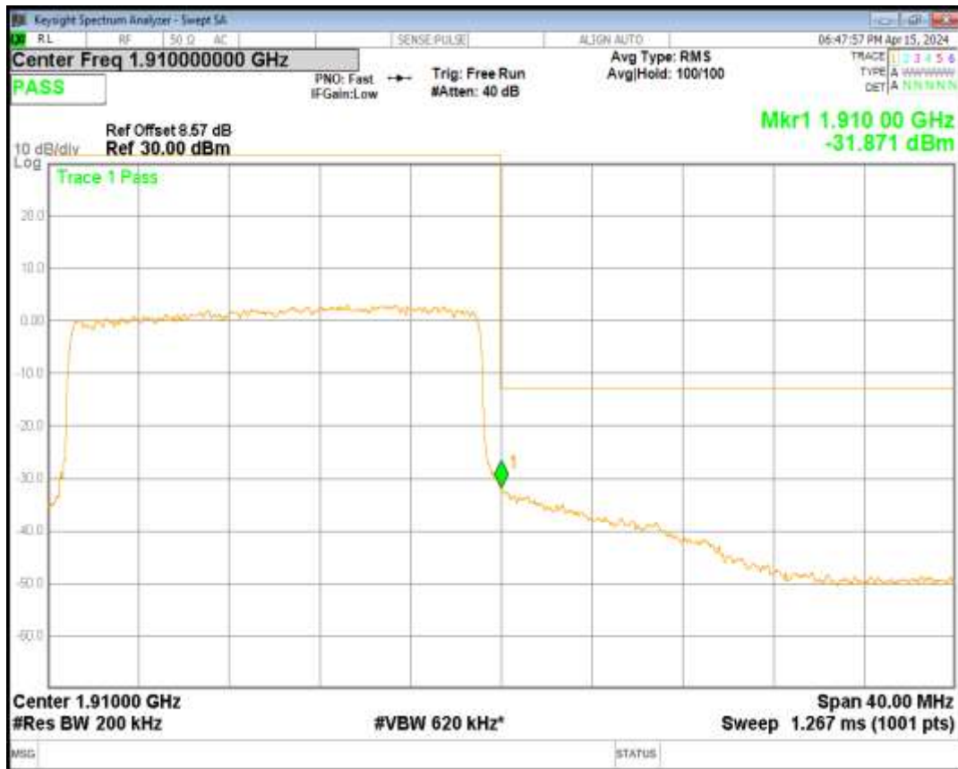
Band5 16QAM BW=1.4MHz Channel=20407 RB Size=6 Position=#0
