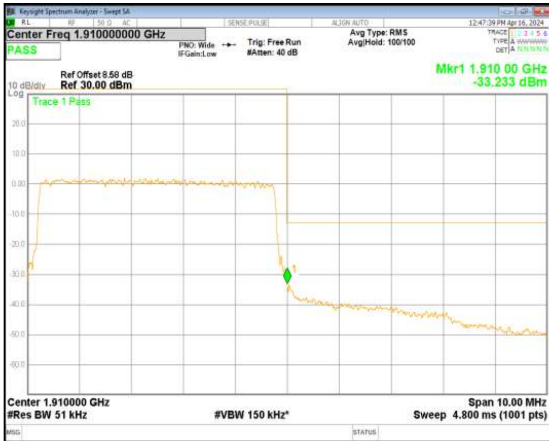
Band2 QPSK BW=1.4MHz Channel=18607 RB Size=6 Position=#0
