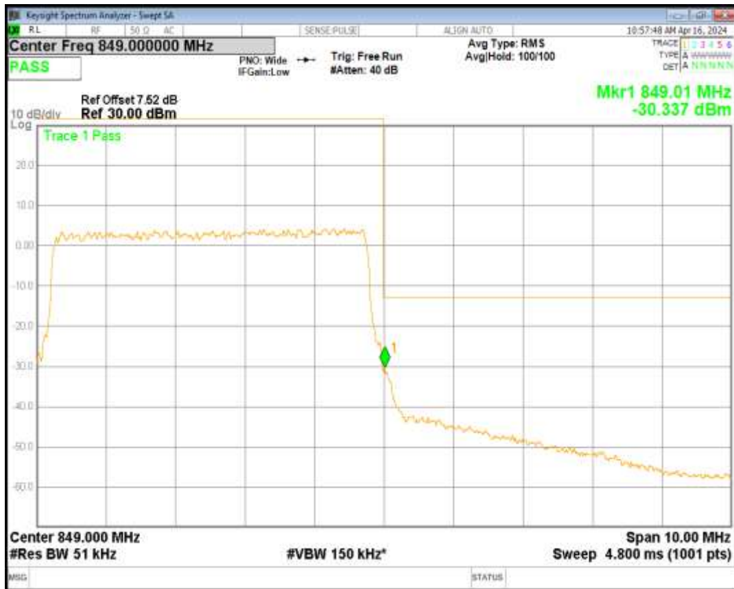
Band5 QPSK BW=10MHz Channel=20450 RB Size=50 Position=#0
