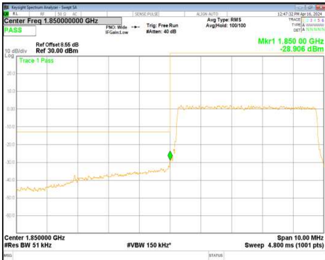
Band2 16QAM BW=5MHz Channel=19175 RB Size=25 Position=#0
