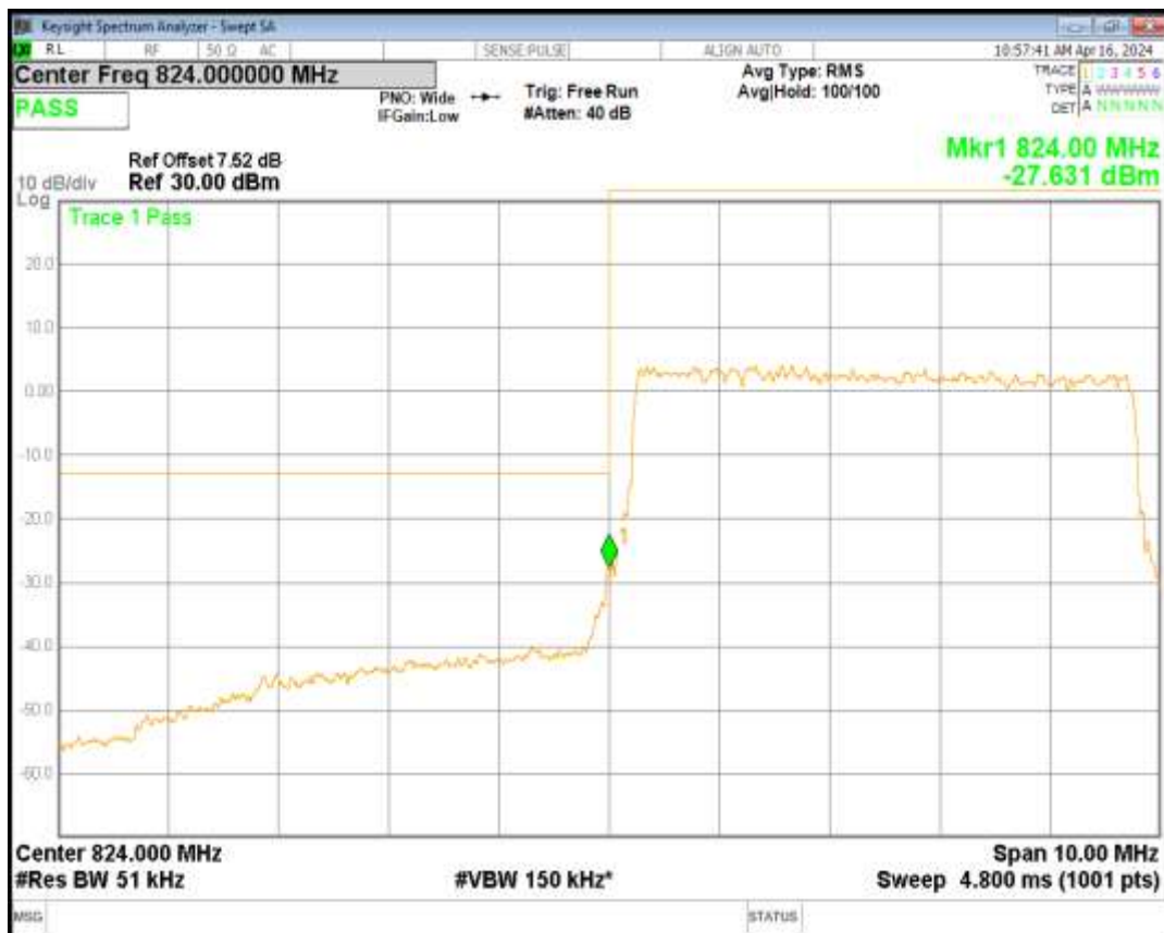
Band5 QPSK BW=5MHz Channel=20625 RB Size=25 Position=#0
