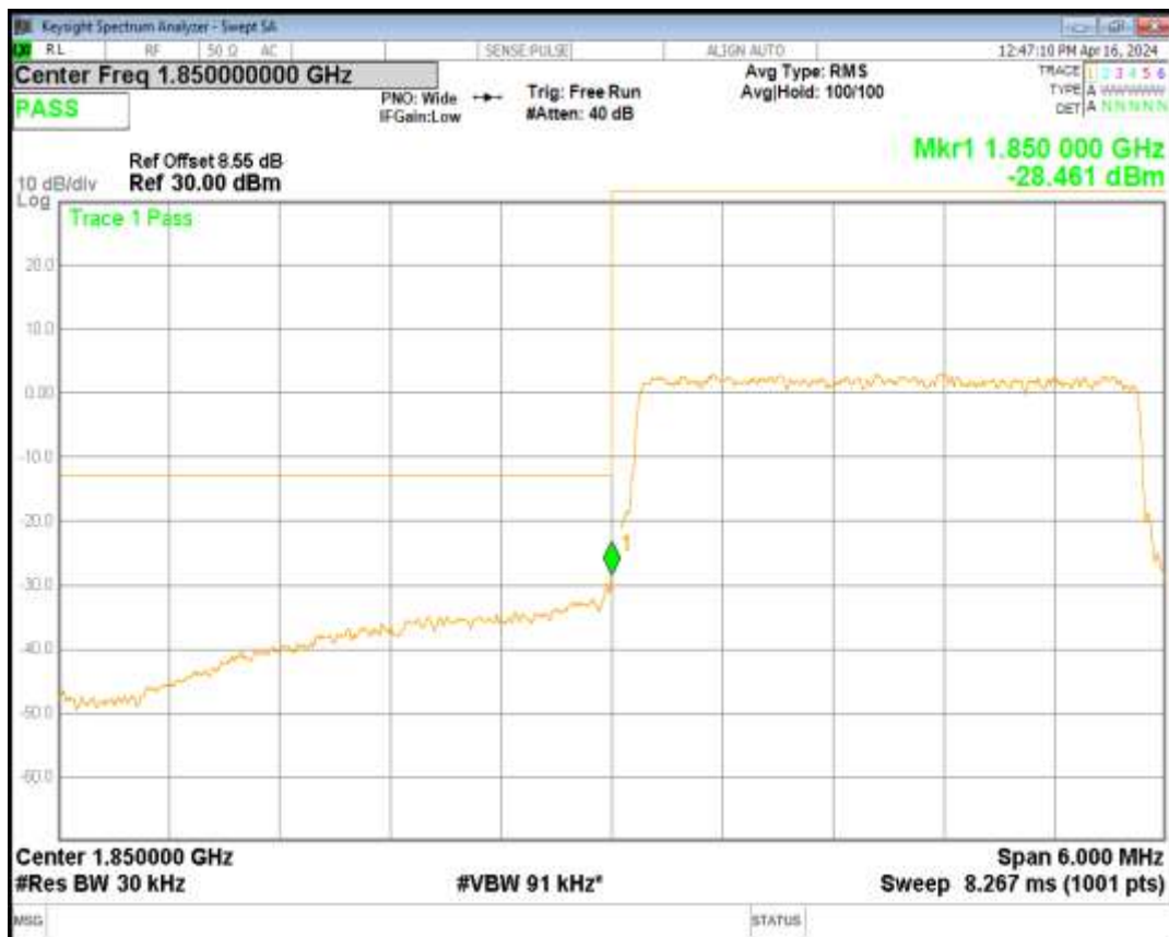
Band2 QPSK BW=3MHz Channel=19185 RB Size=15 Position=#0
