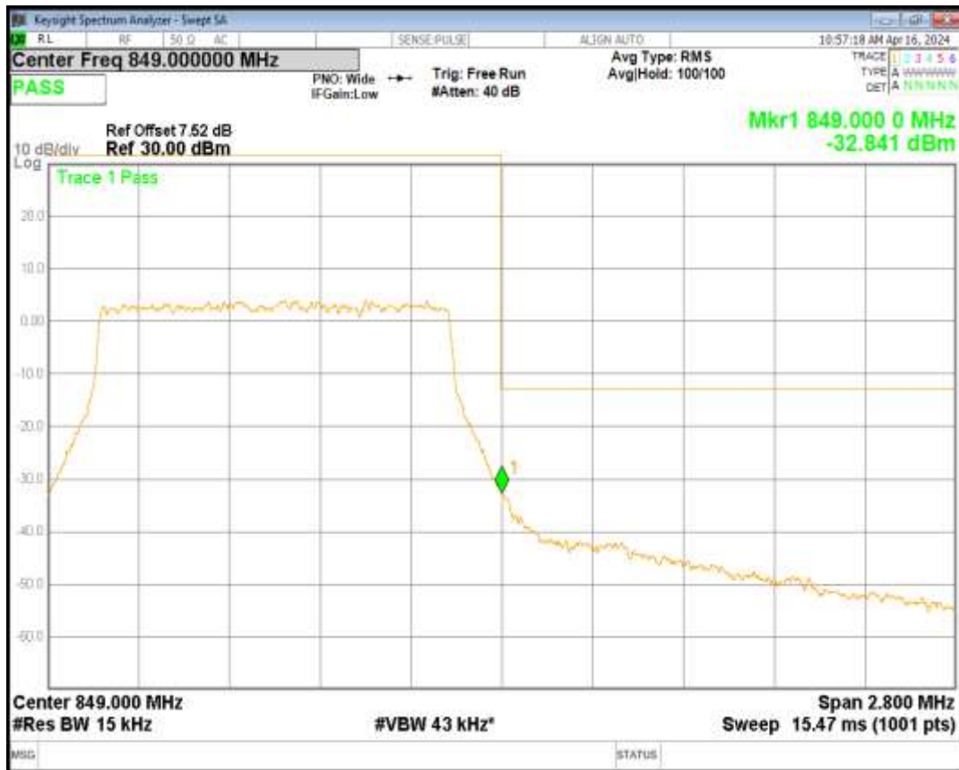
Band5 16QAM BW=3MHz Channel=20415 RB Size=15 Position=#0
