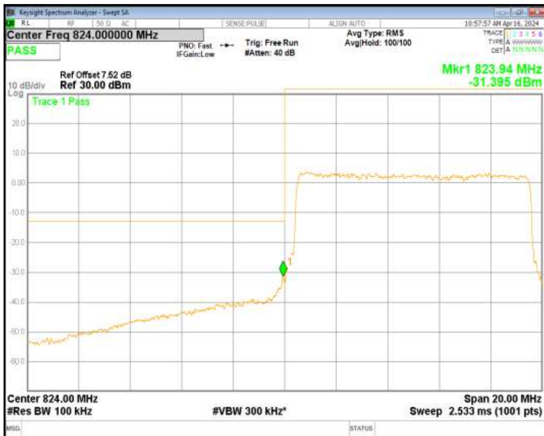
Band5 QPSK BW=10MHz Channel=20600 RB Size=50 Position=#0
