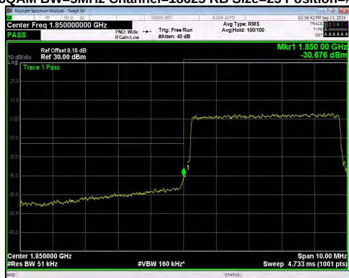
Band2 16QAM BW=5MHz Channel=18625 RB Size=25 Position=#0 Normal
