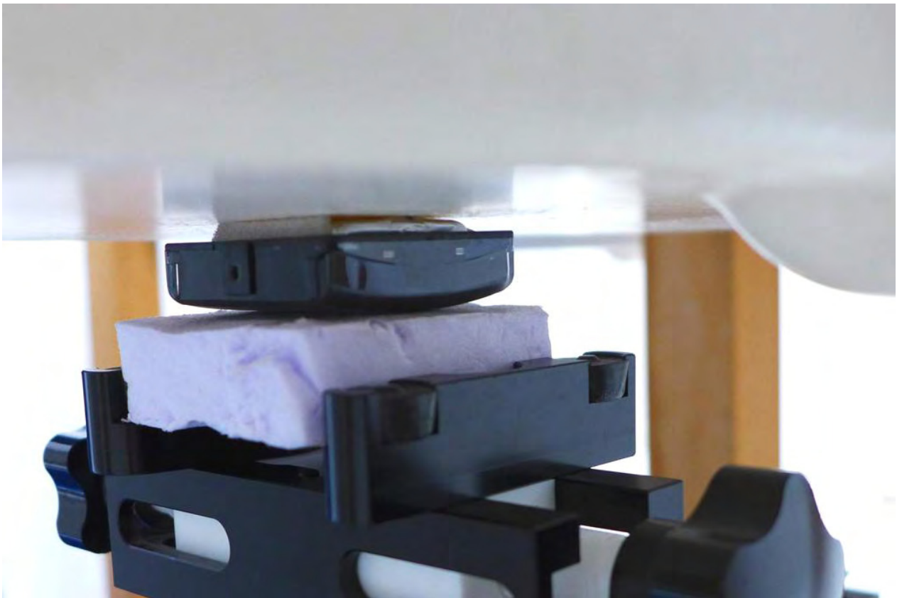
Pic. 8: Configuration 2 – back side, without housing towards the phantom, 0 mm distance
