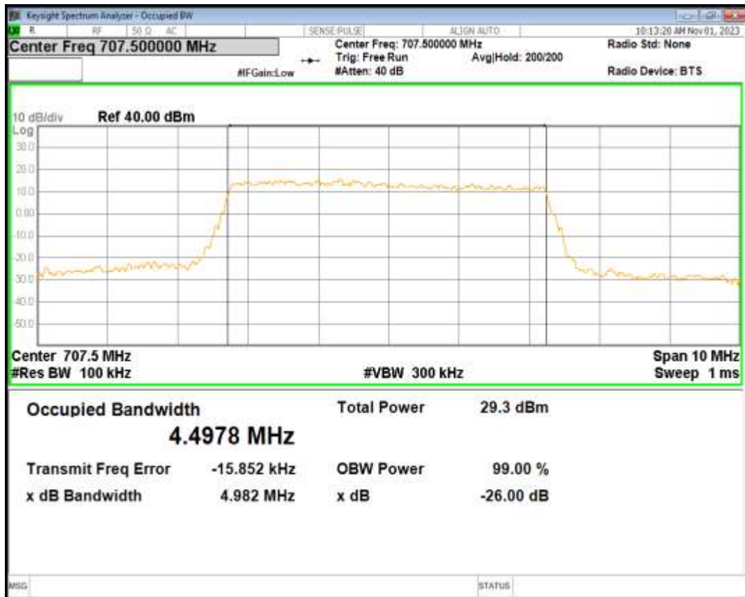
Band12 QPSK BW=5MHz Channel=23155 RB Size=25 Position=#0
