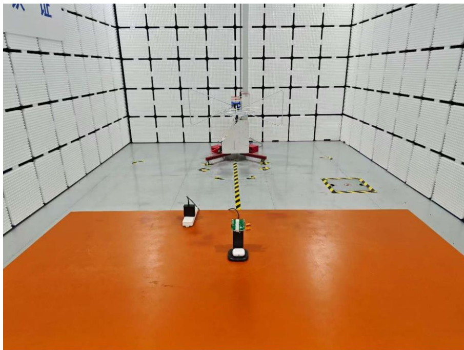
Radiated Emission Above 30MHz
