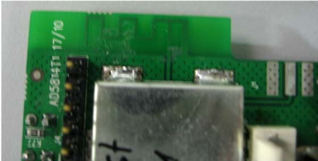
Photograph No.6 RF sensor antenna
