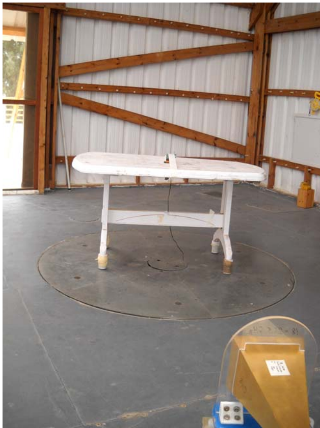
Photograph No.5 Setup for radiated emission measurements at the OATS from 18 to 25 GHz
