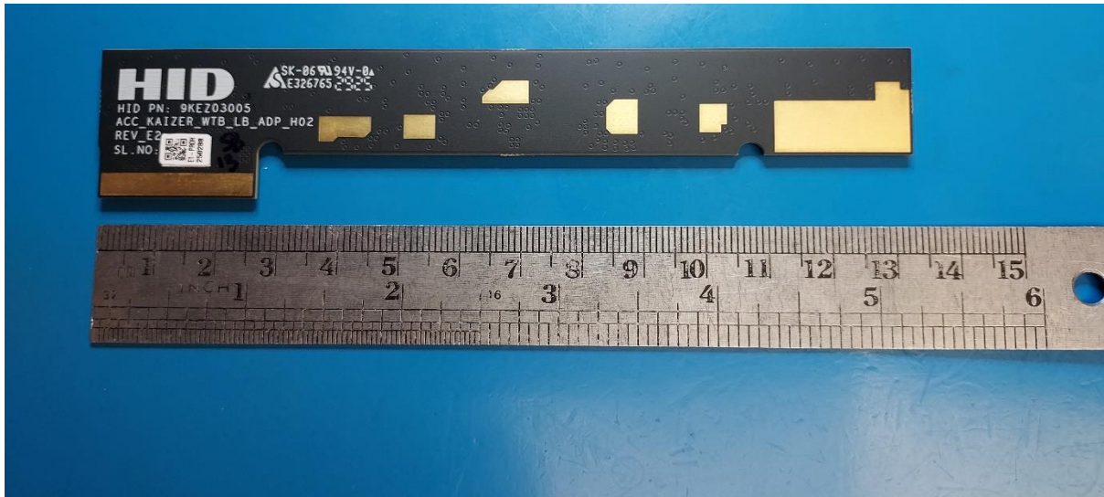
Illumination board top view
