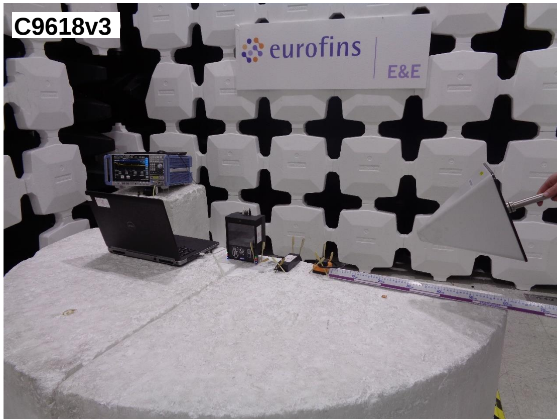
Photo 3: Exploratory Radiated Emissions Maximization, 1GHz to 12.5GHz
