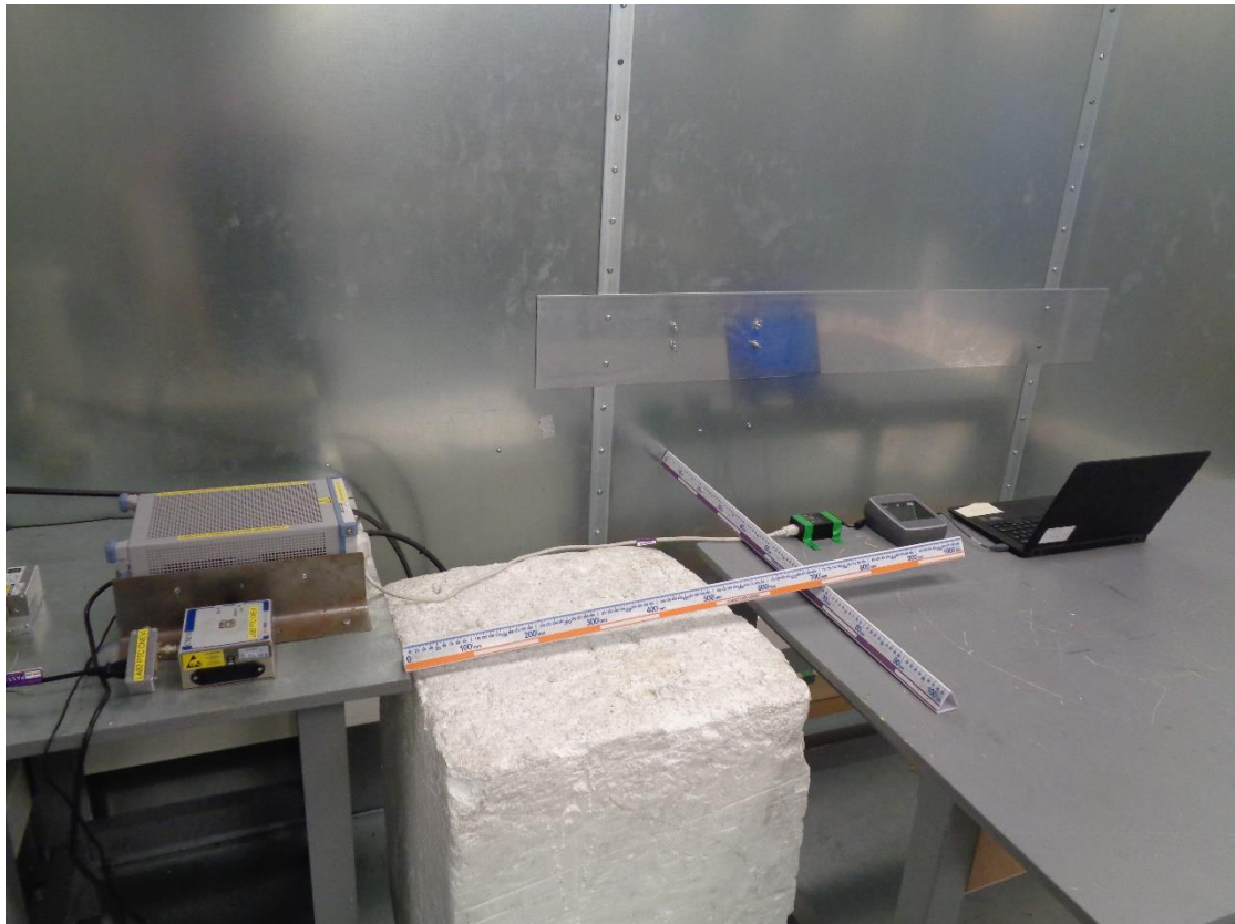
AC Powerline measurements 150kHz to 30MHz
