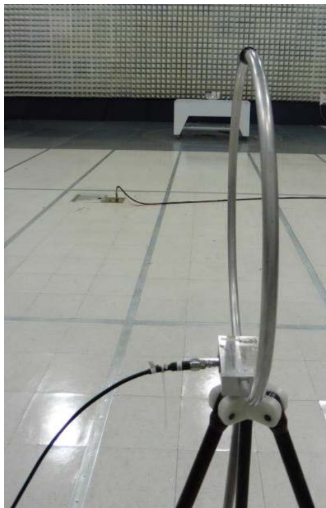
Electromagnetic Radiated Disturbance Setup Photograph
