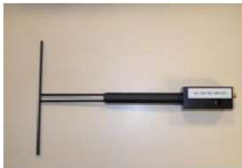
Figure 1 – Satimo COMOSAR Validation Dipole
