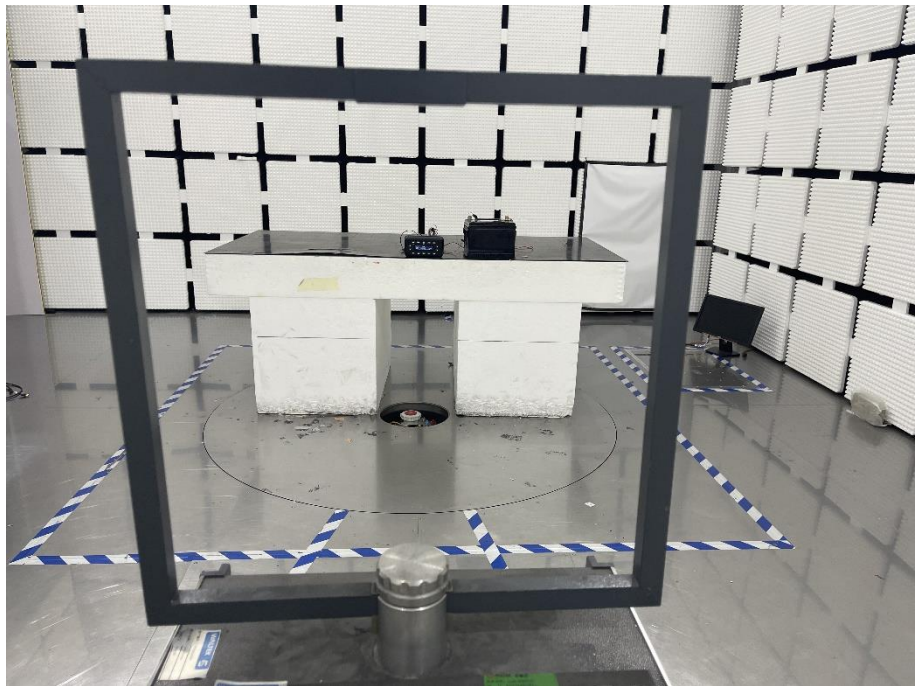
sRadiation Emission Test Setup (Below 30MHz)
