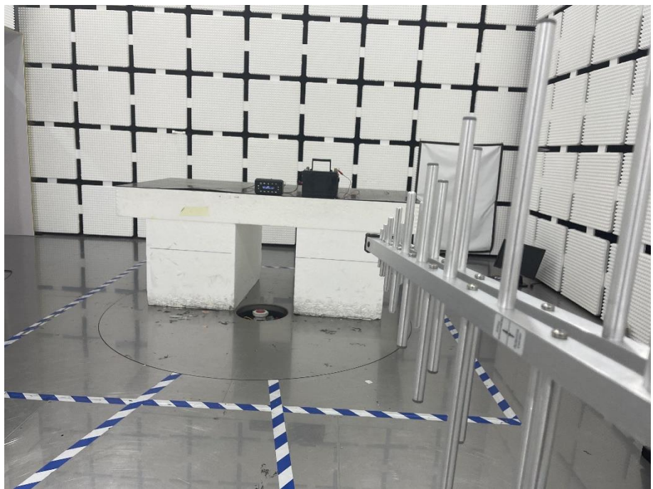
Radiation Emission Test Setup (30MHz to 1GHz)
