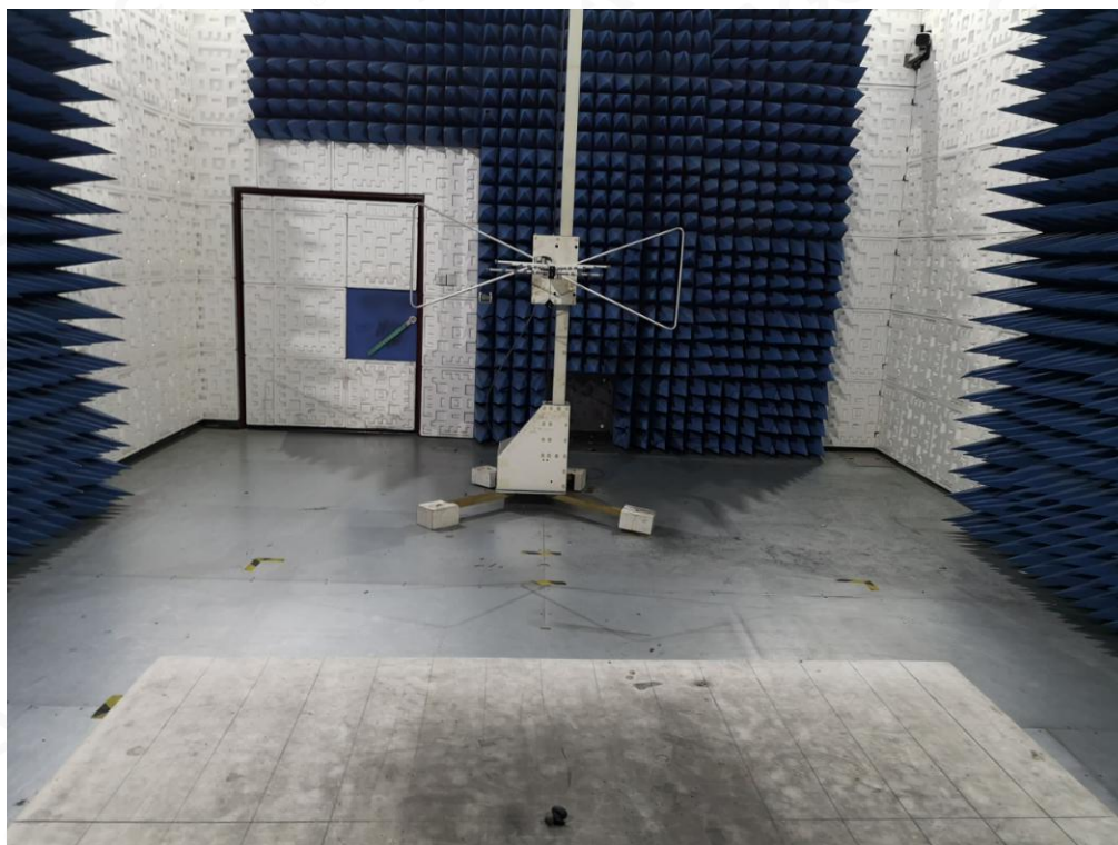
RADIATED EMISSION TEST SETUP ABOVE 1GHZ
