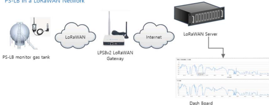
PS-LB in a LoRaWAN Network
