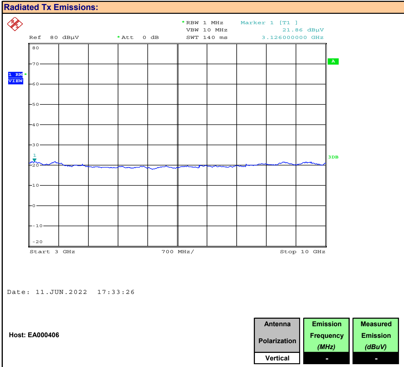
Plot 9.14 – Radiated Tx Emissions, 3 - 10GHz, EA000406, Vertical
