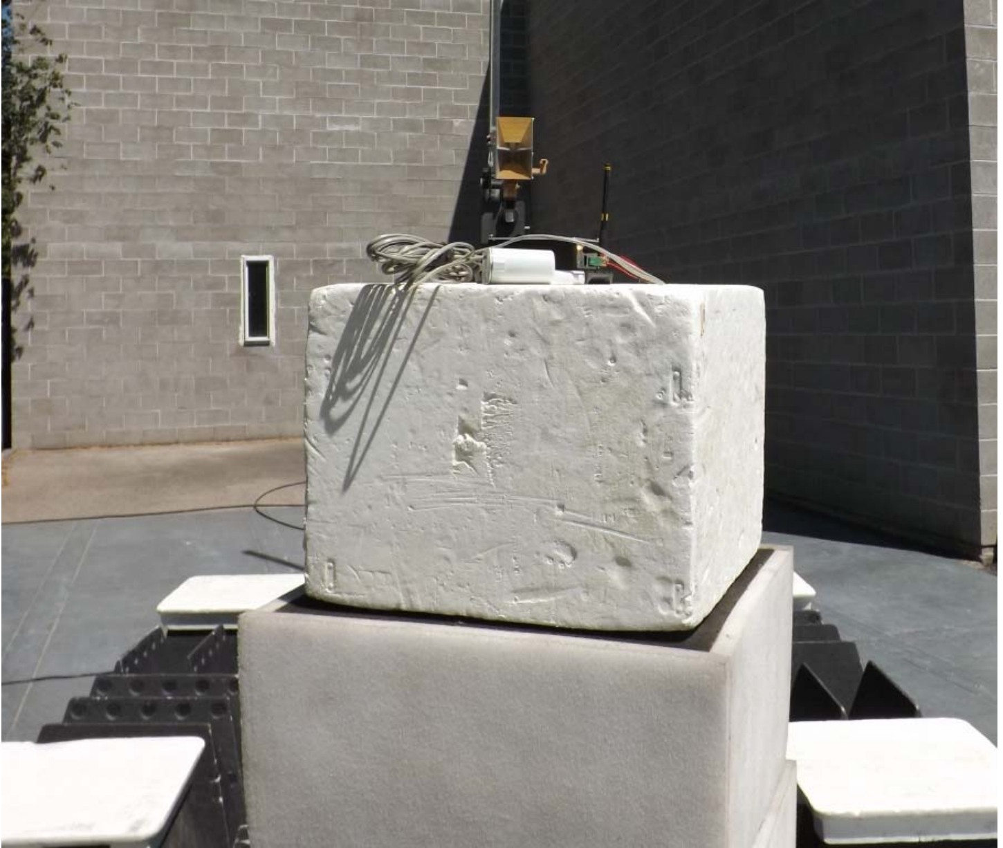
Figure E12.3 – Setup, Radiated Tx, 1 – 10GHz
