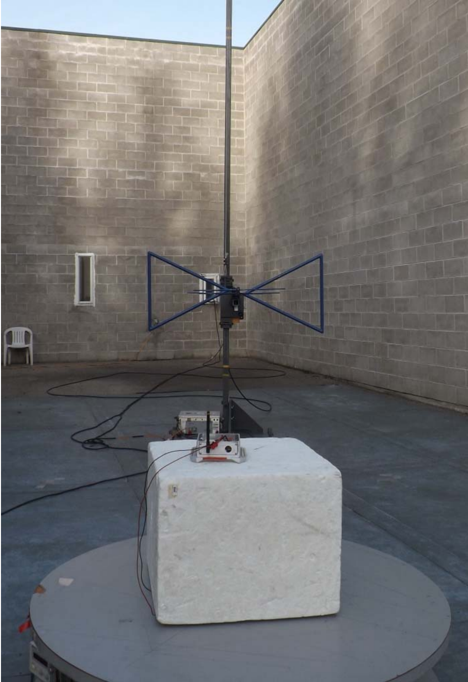
Figure E25.5 – Radiated Measurements 30 – 1000MHz, Horizontal
