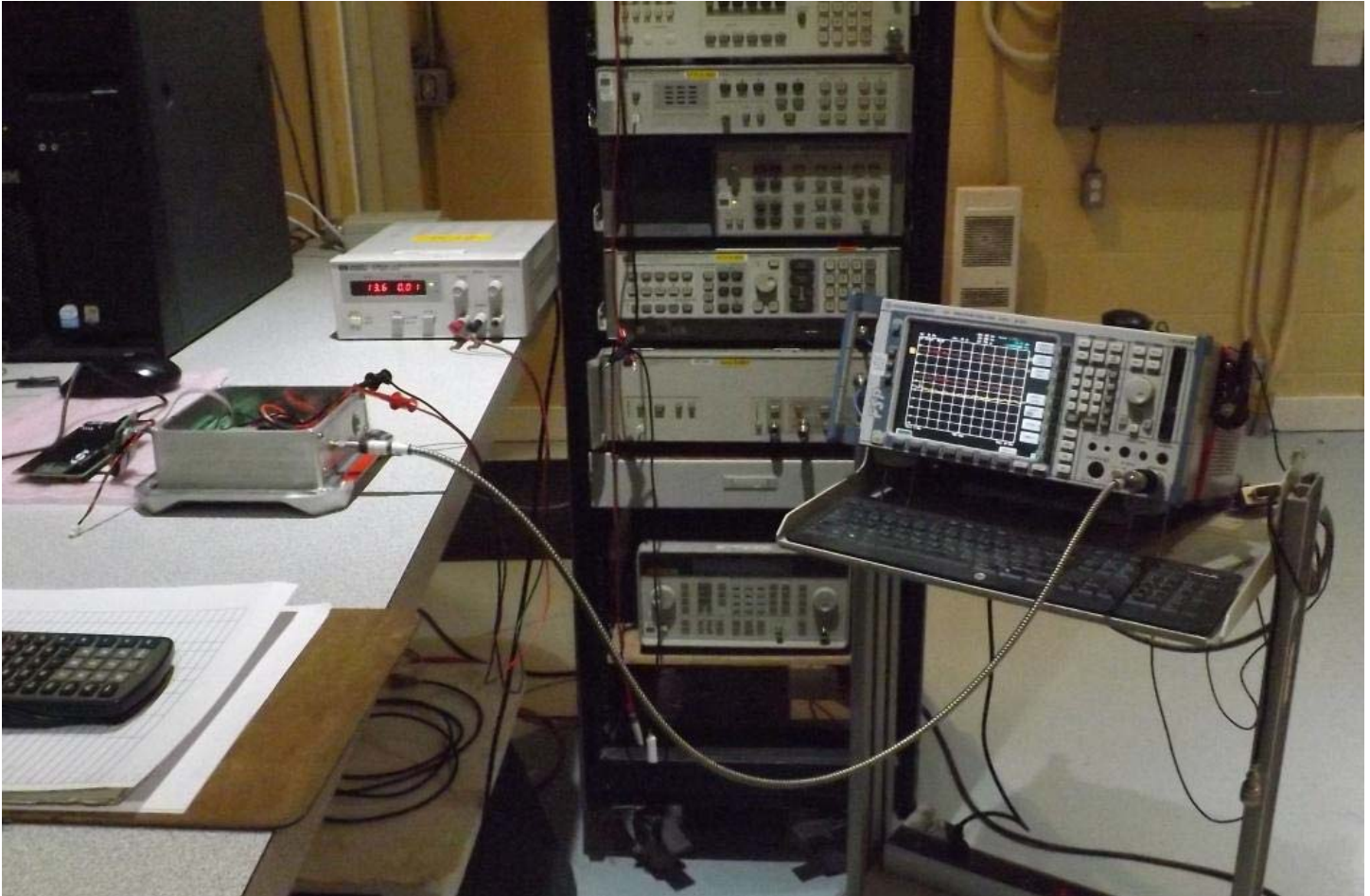
Figure E25.1 – Conducted Measurements
