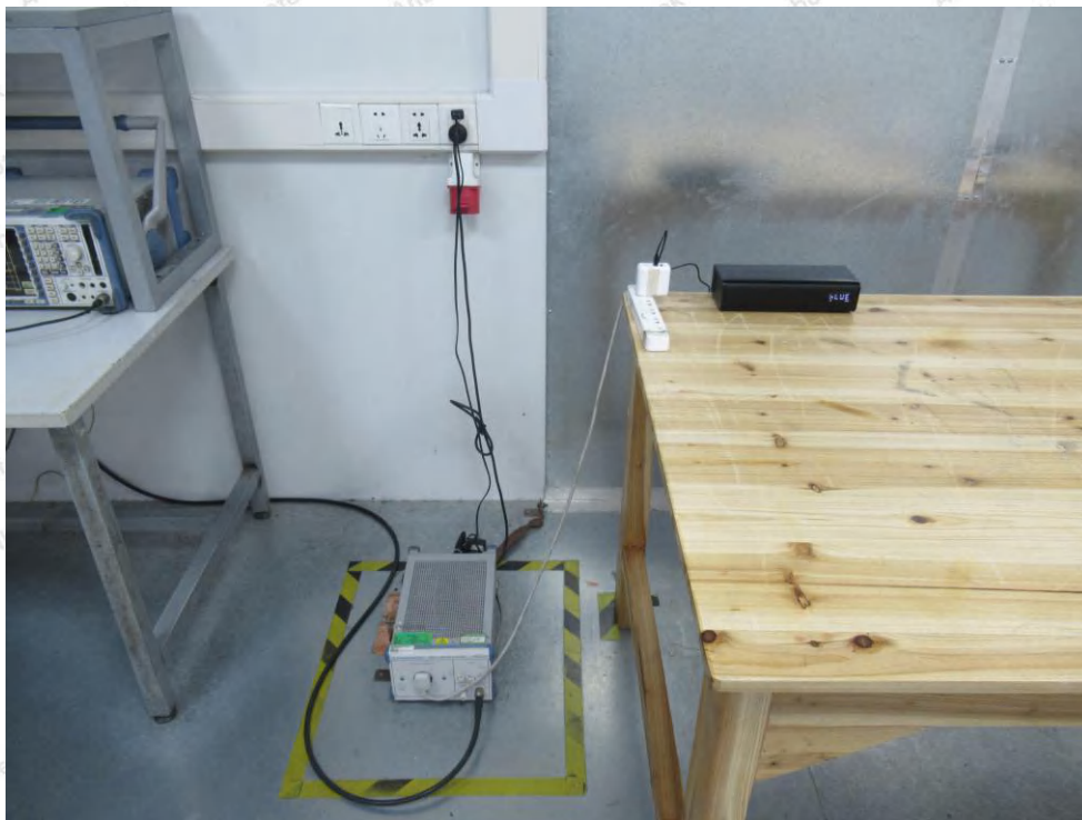
Photo of Conducted Emission Measurement
