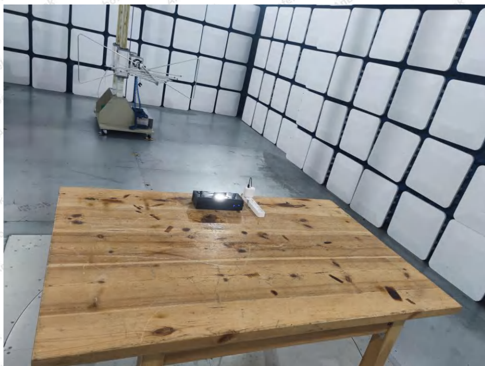
Photo of Radiation Emission Test
