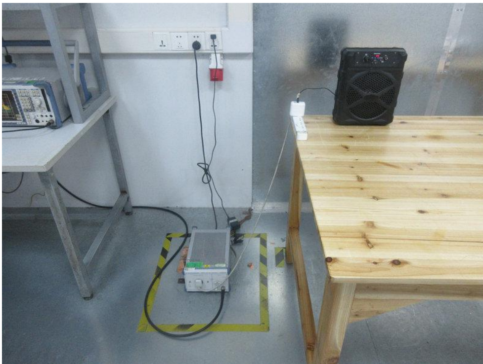
Photo of Power Line Conducted Emission Test
