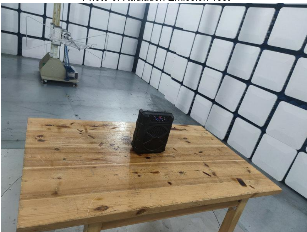
Photo of Radiation Emission Test
