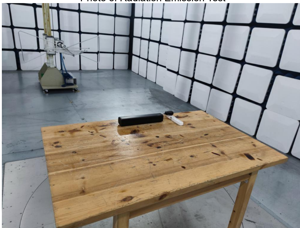
Photo of Radiation Emission Test
