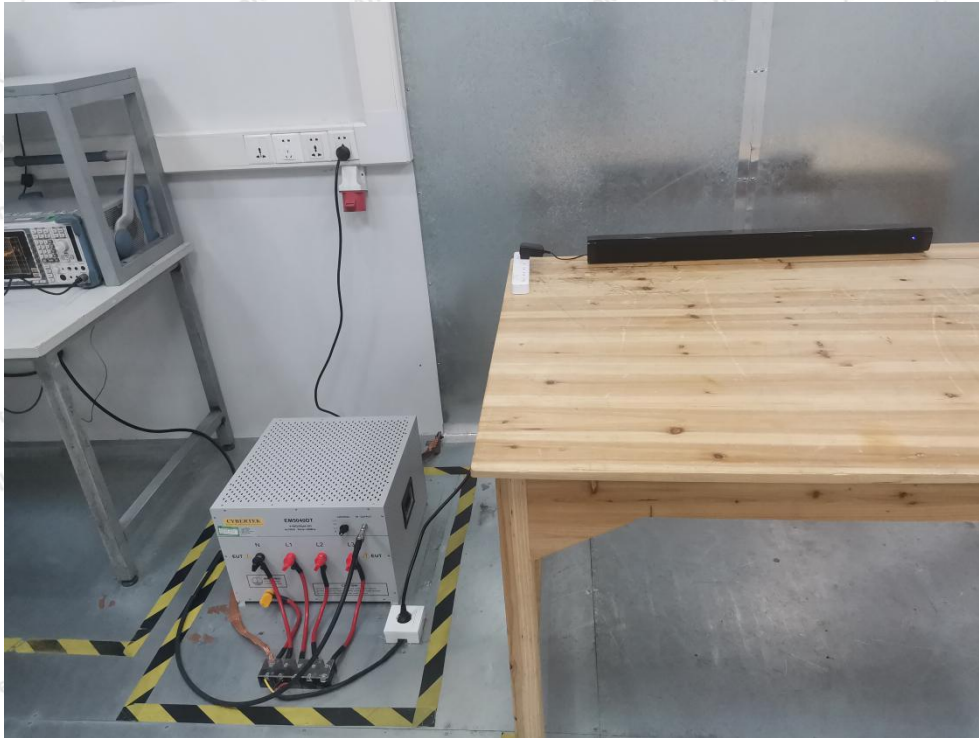
Photo of Conducted Emission Measurement
