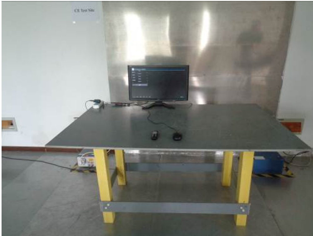
Conducted Emissions Test Setup – Front View
