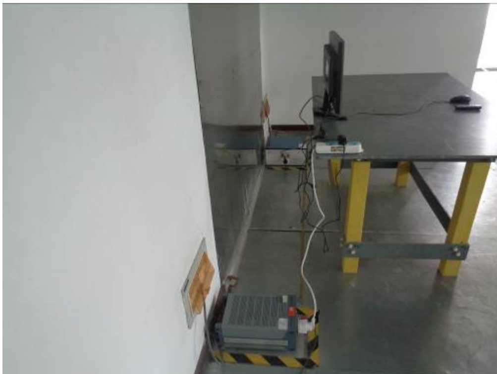
Conducted Emissions Test Setup – Side View
