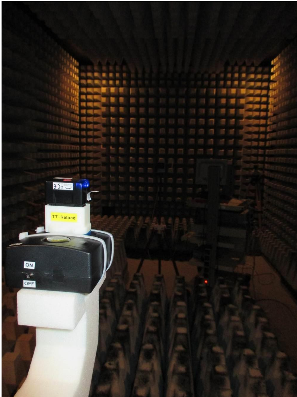
154064_07.jpg: Test setup Device Frog- Radiated emission > 1 GHz (fully anechoic chamber)
