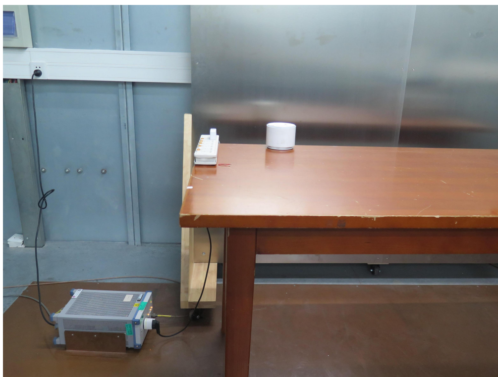
Pic4. Conducted emission (150kHz-30MHz)
