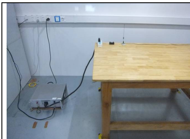
Conducted Emissions Test Setup – Front View
