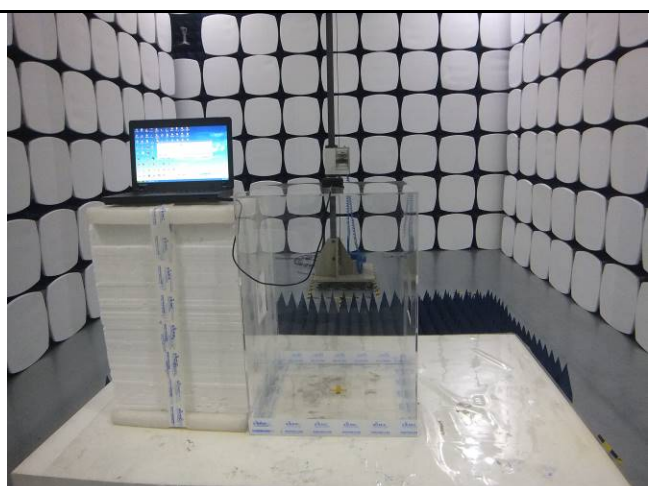
Radiated Emissions Test Setup Above 1GHz
