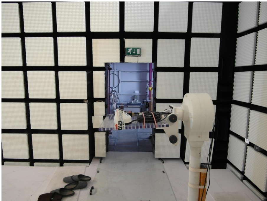
Photo 4: Fully Anechoic Chamber
