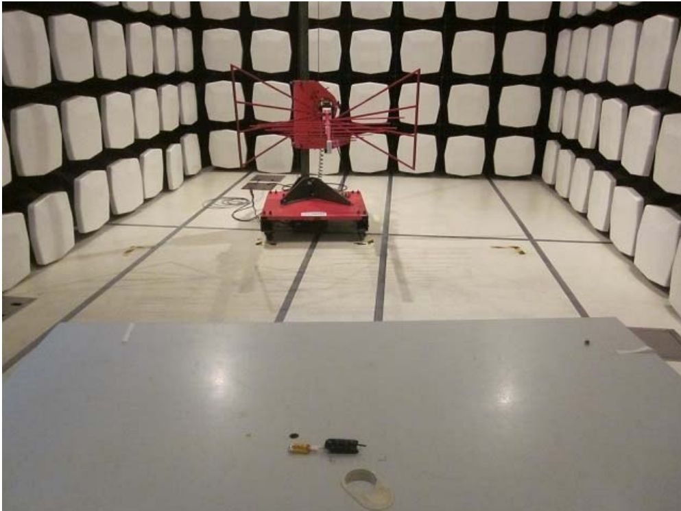
Measurement of Radiated Emission Test Set Up
