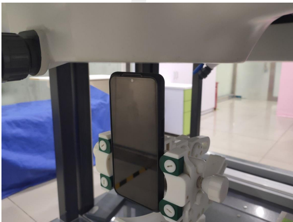
Body Top side(separation distance is 10mm)
